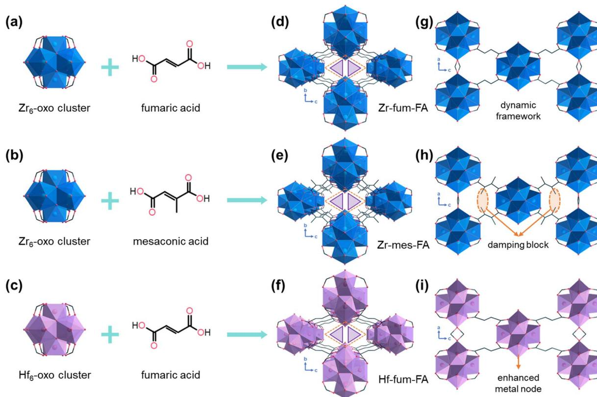
Fig. 2 Component and structure of the three materials. The metal clusters and organic ligands of (a) Zr-fum-FA, (b) Zr-mes-FA, and (c) Hf-fum-FA. (d–f) The double triangle 1D pores along  $a$ -axes and (g–i) the corresponding vertical view along  $b$ -axes of the three materials respectively. Each of the methyl groups on Zr-mes-FA and the  $-\text{CH}$  groups of formate have an occupancy of 0.5. Color scheme: black: C, red: O, blue: Zr, pink: Hf. H atoms are omitted for clarity.
