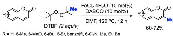
Scheme 18 Iron-catalysed C-3 methylation of coumarins using DTBP.
