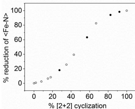
Fig. 5 Relative  $\langle\text{Fe-N}\rangle$  distance reduction (derived from  $100(d(\text{Fe-N})_{[2+2]} - d(\text{Fe-N})_{\text{LS}}) / (d(\text{Fe-N})_{\text{HS}} - d(\text{Fe-N})_{\text{LS}})$ ) versus the degree of [2 + 2] cyclization (estimated from occupancy factors of the cyclobutane derivative) determined at 100 K. First crystal – empty circles; second crystal – filled circles.
