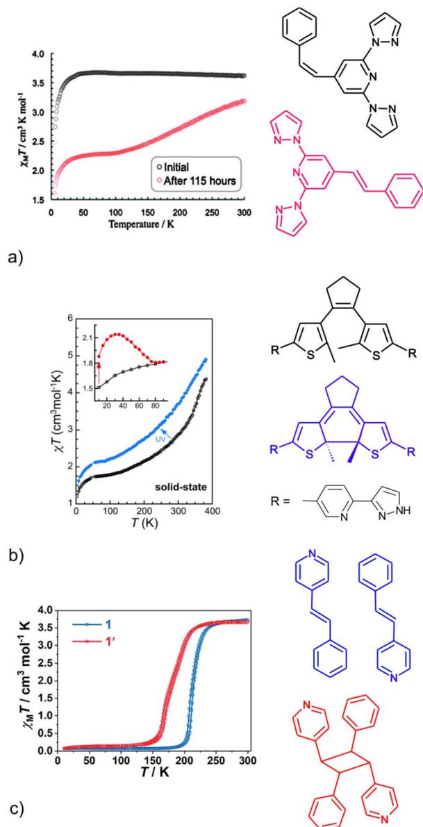
Fig. 1 The effect of *Z*-*E* isomerization of a 4-styrylpyridine based ligand (a), ring closure-opening in a dithienylethene derivative (b) and [2 + 2] cycloaddition of 4-styrylpyridine derivatives (c) on the spin crossover properties of Fe(II) systems. These figures were taken from ref. 24 (a), 29 (b) and 30 (c). On the right side, the structures of ligands (before and after photoconversion) are shown, with the colors corresponding to the temperature dependencies shown on the left side.
