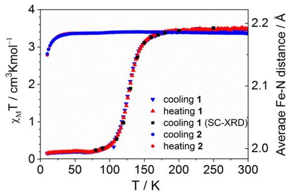
Fig. 2  $\chi_{\text{M}}T(T)$  dependences for **1** (filled triangles) and **2** (filled circles) recorded in cooling (blue) and heating (red) modes. Black squares denote average Fe–N distances determined during cooling. Temperature scan rate: 1 K min<sup>-1</sup>. Applied magnetic field: 1 T.
