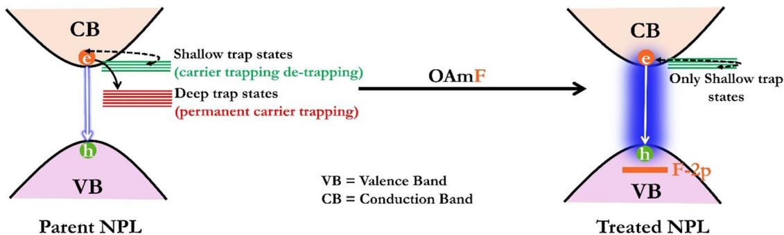
**Scheme 2** Schematic representation of oleylammonium fluoride post-synthetic treatment on CsPbBr<sub>3</sub> NPLs to reveal the enhancement in PLQY by passivation of deep trap states.
