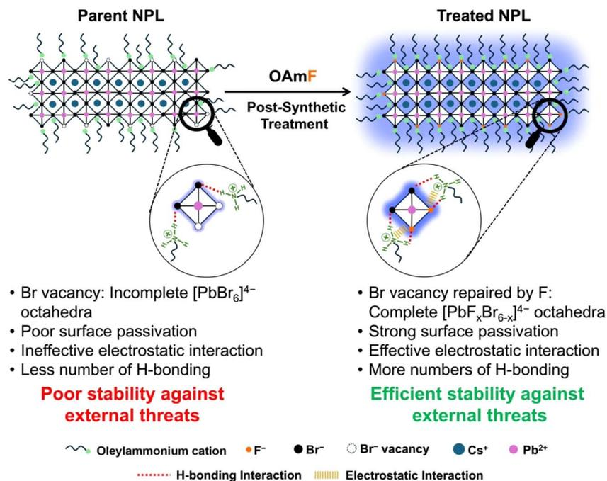
**Scheme 3** Plausible mechanism for the enhanced stability of treated NPLs against external perturbations like heat, UV irradiation, water and atmospheric conditions after post-synthetic treatment with oleylammonium fluoride (OAmF).
