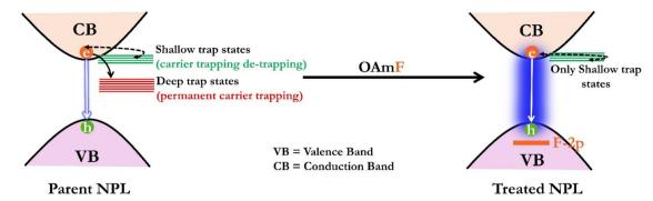
Scheme 2 Schematic representation of olevlammonium fluoride post-synthetic treatment on CsPbBr<sub>3</sub> NPLs to reveal the enhancement in PLQY by passivation of deep trap states.
