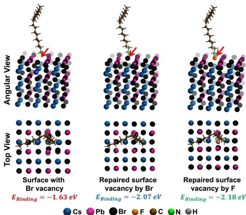
Fig. 6 Angular and top views of optimized CsPbBr<sub>3</sub> crystal slabs (100) with one Br vacancy (left panel), Br vacancy is filled by a bromine atom (middle panel) and Br vacancy is filled by a fluorine atom (right panel), in the presence of oleylammonium ligand.
