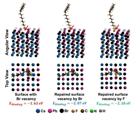
Fig. 6 Angular and top views of optimized  $CsPbBr_3$  crystal slabs (100) with one Br vacancy (left panel), Br vacancy is filled by a bromine atom (middle panel) and Br vacancy is filled by a fluorine atom (right panel), in the presence of oleylammonium ligand.
