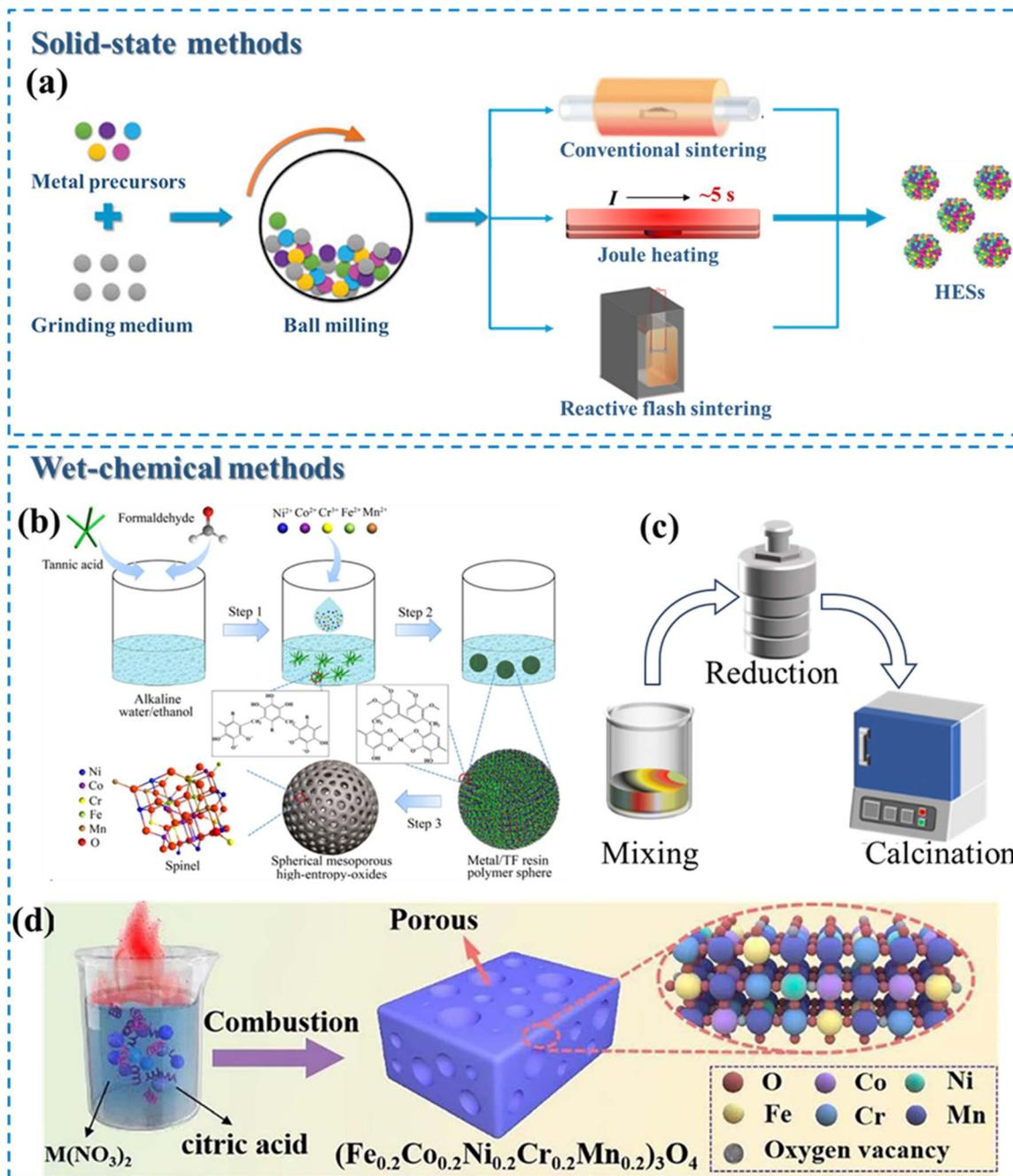
Fig. 3 Conventional methods for HES synthesis. (a) Synthetic procedures of different solid-state methods. Reproduced with permission.<sup>41</sup> Copyright 2022, John Wiley and Sons. Wet-chemical methods: (b) sol-gel method. Reproduced with permission.<sup>67</sup> Copyright 2020, American Chemical Society. (c) Hydro-/solvothermal methods. (d) Solution combustion synthesis. Reproduced with permission.<sup>68</sup> Copyright 2023, Elsevier.
