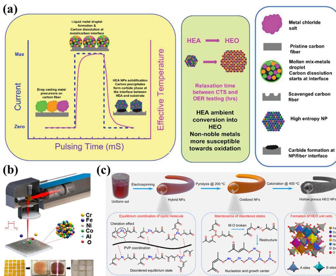
Fig. 4 Emerging methods for HES synthesis. (a) Schematic illustration of the carbothermal shock (CTS) synthesis process within mS pulse intervals.<sup>80</sup> (b) Laser-based shock methods. Reproduced with permission.<sup>81</sup> Copyright 2021, American Chemical Society. (c) Electrospinning. Reproduced with permission.<sup>82</sup> Copyright 2024, American Chemical Society.
