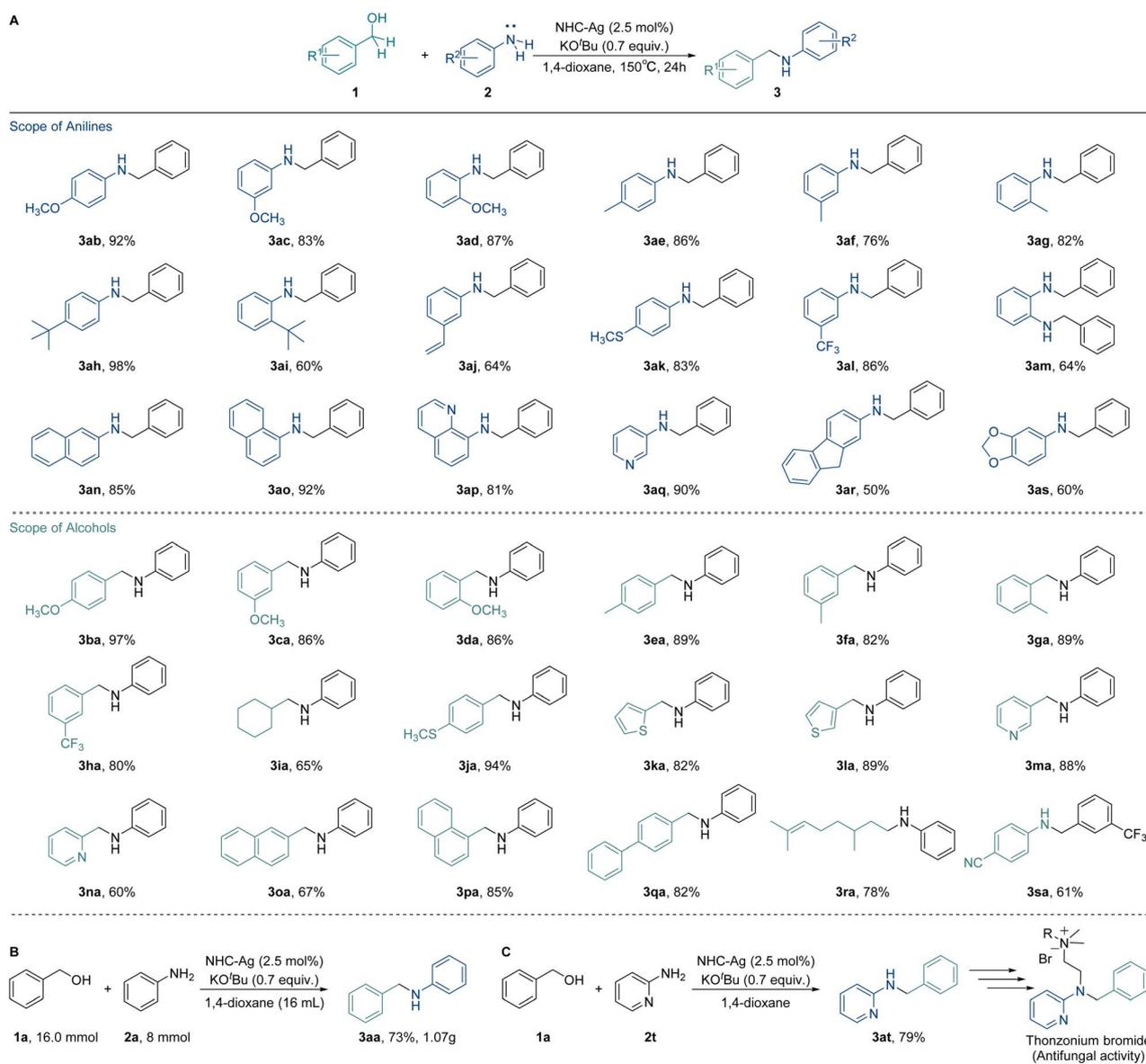
Fig. 5 Substrate scope of silver catalyzed *N*-alkylation and applications. (A) Scope of substrates. Optimal conditions: anilines (**2**, 0.5 mmol), alcohols (**1**, 1.0 mmol), NHC-Ag (2.5 mol%), KO<sup>t</sup>Bu (0.7 equiv.), 1,4-dioxane (1 mL), 150 °C, and 24 h. (B) Gram-scale reaction. Conditions: aniline (**2a**, 8.0 mmol), benzyl alcohol (**1a**, 16.0 mmol), NHC-Ag (2.5 mol%), KO<sup>t</sup>Bu (0.7 equiv.), 1,4-dioxane (16 mL), 150 °C, and 24 h. (C) Synthetic application.
