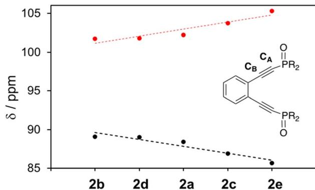
Fig. 5  $^{13}\text{C}$  NMR resonances of phosphine oxide analogues **2a–2e** revealing the polar nature of the alkyne carbons,  $\text{C}_A$  (black) and  $\text{C}_B$  (red), the magnitude of which is enhanced in the presence of electron withdrawing substituents.
