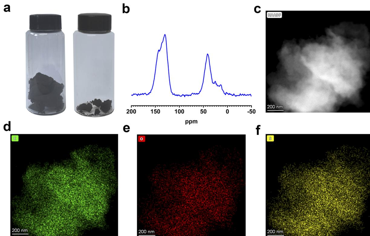
Fig. 2 (a) Optical photos of volume change for porous precursor before (right) and after (left) thermal treatment. (b) Solid-state  $^{13}\text{C}$  CP-MAS NMR spectrum of the resulting polymer. (c–f) High-angle annular dark field (HAADF) mapping images of the resulting polymer.
