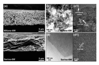
Fig. 5 The cross-sectional SEM images of (a) fresh MXene and (b) serine-functionalized MXene after 6 weeks of aging. TEM images of (c) fresh MXene and (d) serine-functionalized MXene along with their (c1 and d1) HR-TEM images after 6 weeks of aging.
