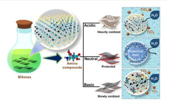
Fig. 1 Graphical representation of MXene dispersion stabilized using different kinds of amino acids.
