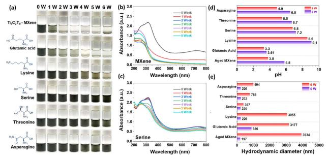
Fig. 2 (a) The visual appearance of pristine MXene and amino acid-functionalized MXene dispersion after different time intervals. UV-vis analysis of (b) fresh MXene and (c) amino acid-functionalized MXene dispersion. The change in (d) pH and (e) hydrodynamic diameter after 0 and 6 weeks of fresh MXene and amino acid-functionalized MXene dispersion.
