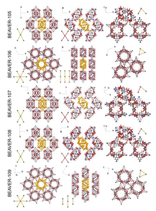
$\textbf{Fig. 4} \quad \textbf{Crystal packing of the five Mo(v)-MOP solvatomorphs viewed in two orthogonal planes. The planes correspond to those shown in Fig. 3 in a solvator of the five Mo(v)-MOP s$ 3D. Arrays of intermolecular MOP···MOP hydrogen bonds between neighboring Mo(v)-MOP molecules are shown to the right. Color code: C, light gray; H, dark gray, Mo, green; N, blue; O, red. The molecules and the H-bonds of interest are emphasized in orange.
