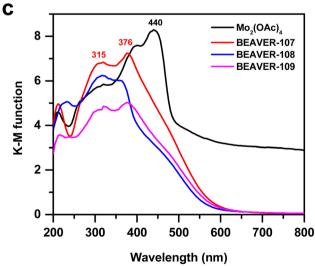
Fig. 2 Spectroscopic features of the Mo(v)-MOP molecule. (a) X-ray photoelectron spectra of BVR-107. (b) Fourier-transform infrared and (c) ultraviolet-visible spectra of  $Mo_2(OAc)_4$ , BVR-107, BVR-108, and BVR-109. All sets of spectra were recorded on the respective solids.
