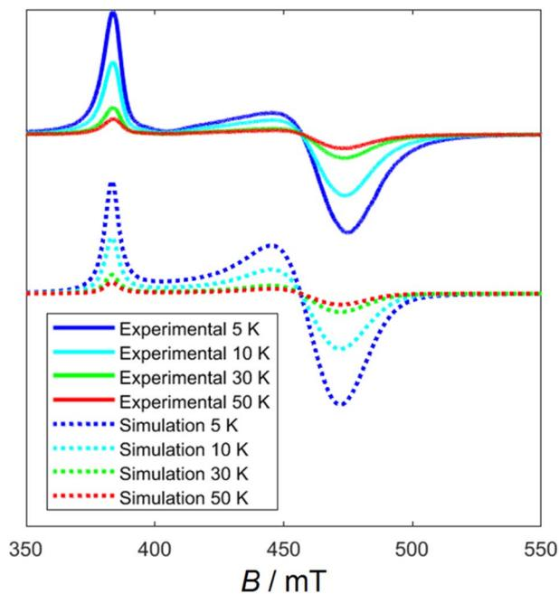
Fig. 4 Experimental X-band EPR spectra (continuous lines) and their simulations (dotted lines) for  $[\text{EuRad}(\text{NO}_3)_3]$  at the temperatures of 5, 10, 30 and 50 K obtained using parameters and Hamiltonian reported in the text.
