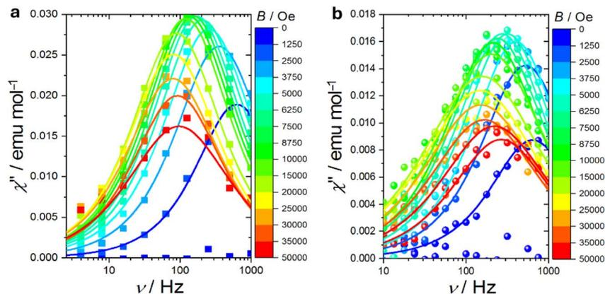
Fig. 8 Field evolution of the imaginary component of the magnetic susceptibility for [LnRad(NO<sub>3</sub>)<sub>3</sub>] at  $T = 5$  K: (a) Lu; (b) Eu. The lines are the best fits discussed in the text.
