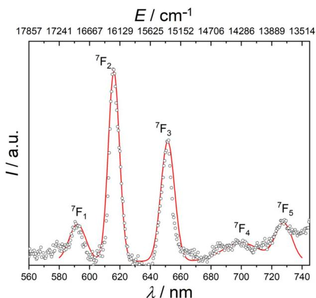
Fig. 2 Room temperature photoluminescence emission spectrum for solid [EuRad(NO<sub>3</sub>)<sub>3</sub>] at excitation wavelength of 397 nm. The red line is a simple fit using a sum of five gaussian curves.
