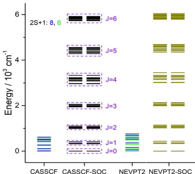
Fig. 5 The lowest spin multiplets (seven octets and sextets) calculated for  $[\text{EuRad}(\text{NO}_3)_3]$  at SA-CASSCF(7,8) (CASSCF) and SA-CASSCF(7,8)/NEVPT2 (NEVPT2) and SO-multiplets after account of SOC at QDPT level (CASSCF-SOC and NEVPT2-SOC). Kramers doublets appearing after account of SOC are roughly presented as a result of interaction between  $\text{Eu}^{3+}$  states with assigned full moment  $J$  (purple) and ligand doublet state interaction.
