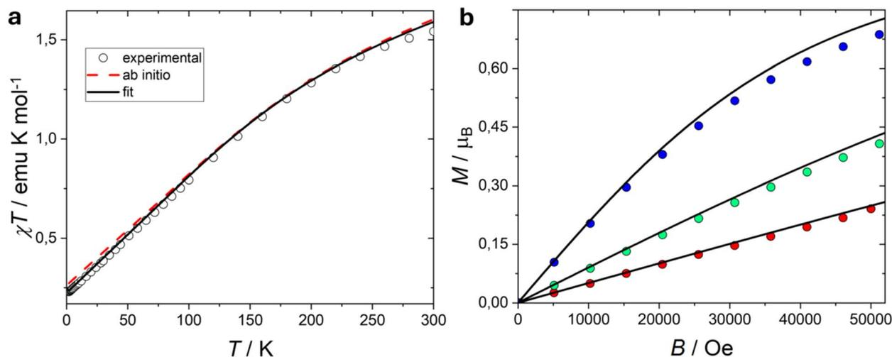
**Fig. 3** Magnetic behaviour of  $[\text{EuRad}(\text{NO}_3)_3]$ : (a) temperature dependence of  $\chi T$  product at  $B = 0.1$  T; (b) magnetization curve measured at 1.8 K (blue), 5 K (green) and 10 K (red). Black continuous lines are the best fits obtained with the model described in the text. The dashed red line is the SA-CASSCF(7,8)/NEVPT2/QDPT calculated  $\chi T$  curve.
