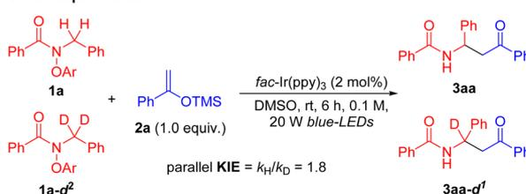
Scheme 7 Mechanistic experiments. (a) Radical trapping experiment with the *N*-allyl amide **1u**. (b) Intramolecular deuterium isotope effect experiment. (c) Parallel KIE experiments.
