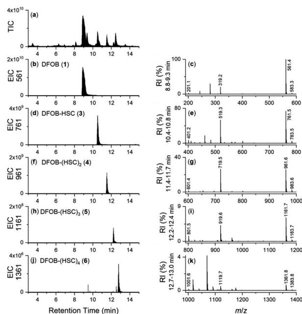
Fig. 2 LC-MS traces from solutions of **1** and **2** with  $\text{MgCl}_2$  and ATP, incubated ( $37^\circ\text{C}$ , 2 h, pH 8) in the presence of *StDesD*, as detected by TIC (a), or shown as an EIC with values set to report the  $[\text{M} + \text{H}]^+$  adducts of (b) **1**, (d) **3**, (f) **4**, (h) **5**, or (j) **6**, with signature regions of the MS fragmentation pattern aligned at right (c, e, g, i and k).
