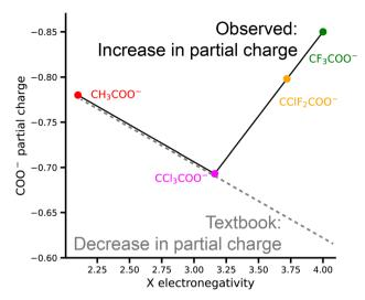
Fig. 2 Charge densities of carboxylate groups in substituted acetates. The relationship between the mean Pauling electronegativity<sup>18</sup> of the alpha substituent(s) on the carboxylate group. This value comes from the summation of the partial charges of the carboxylate carbon, and the two oxygen atoms as shown in Fig. 1f/g. DDEC6 charges calculated using MP2/aug-cc-pVQZ. The COO<sup>-</sup> axis has been inverted to aid in understanding.
