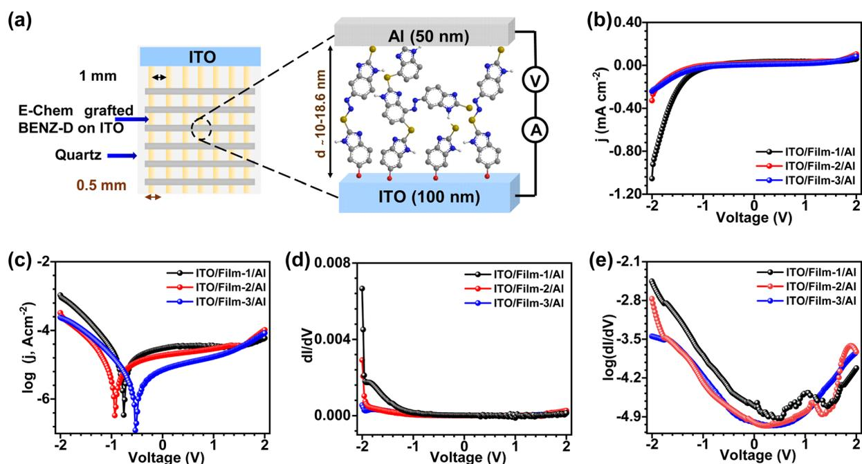
Fig. 3 Fabrication of ITO/BENZ/Al MJs of varying thicknesses followed by *I*-*V* characterization. (a) Illustration of ITO/BENZ/Al molecular junctions, and zoomed-in side view of an MJ. Comparison of (b) *j*-*V* plots, (c)  $\log j$ -*V*, (d)  $dI/dV$  vs. *V*, and (e)  $\log(dI/dV)$  vs. *V* plots of ITO/Film-1/Al to ITO/Film-3/Al MJs; *j* is the current density in  $\text{Amp cm}^{-2}$ .
