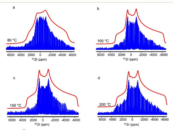
Fig. 4 Experimental 1D  $^{91}$ Zr WURST-QCPMG NMR spectra (in blue) of UiO-66 submitted to steam flow during 7 days at (a) 80, (b) 100, (c) 150 and (d) 200  $^{\circ}$ C recorded under static conditions at  $B_0 = 18.8$  T and 140 K along with their simulated envelope (in red).
