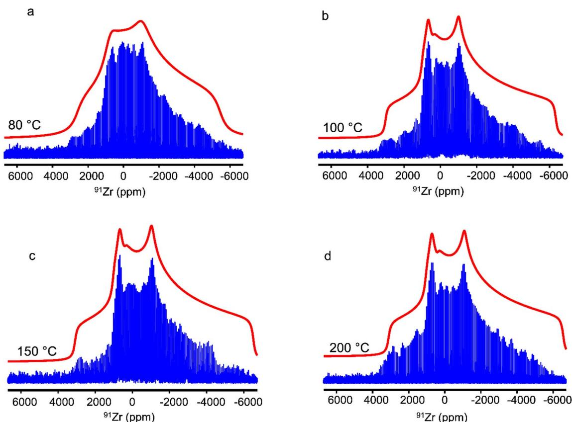
Fig. 4 Experimental 1D <sup>91</sup>Zr WURST-QCPMG NMR spectra (in blue) of UiO-66 submitted to steam flow during 7 days at (a) 80, (b) 100, (c) 150 and (d) 200 °C recorded under static conditions at  $B_0 = 18.8$  T and 140 K along with their simulated envelope (in red).
