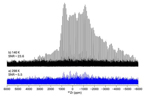
Fig. 2 1D  $^{91}$ Zr WURST-QCPMG NMR spectra of activated UiO-66 recorded at  $B_0 = 18.8$  T and (a) 298 and (b) 140 K under static conditions.
