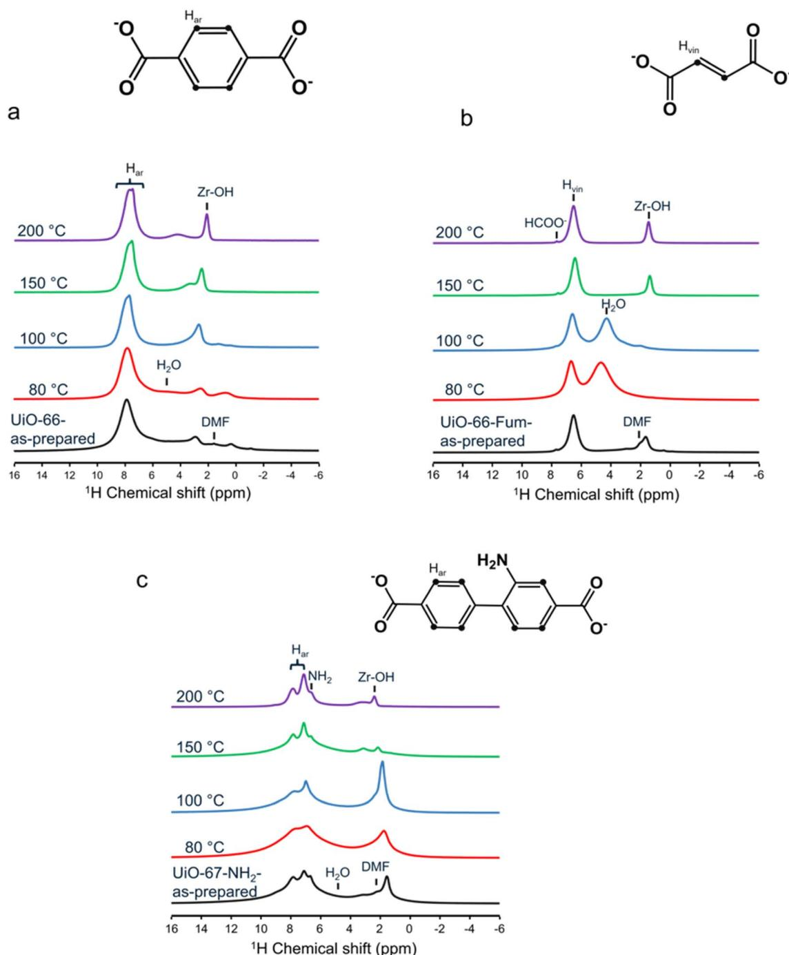
Fig. 1 1D <sup>1</sup>H NMR spectra of the (a) UiO-66, (b) UiO-66-Fum and (c) UiO-67-NH<sub>2</sub> MOFs: as-prepared materials (black), and after steam flow treatment at 80 (red), 100 (blue), 150 (green) and 200 °C (purple).
