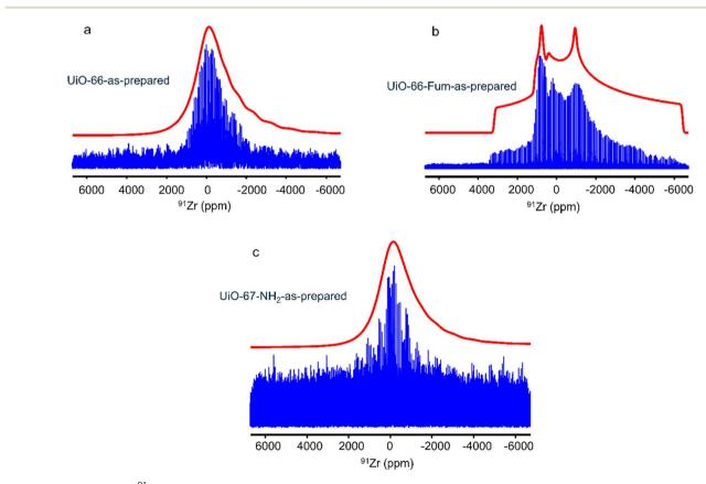
Fig. 3 Experimental 1D  $^{91}$ Zr WURST-QCPMG NMR spectra (in blue) of the as-prepared (a) UiO-66, (b) UiO-66-Fum and (c) UiO-67-NH<sub>2</sub> recorded under static conditions at  $B_0 = 18.8$  T and 140 K along with their simulated envelope (in red).
