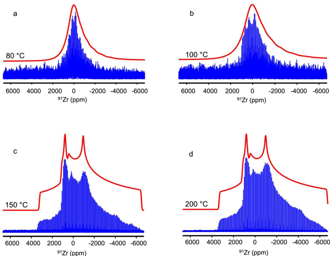
Fig. 5 Experimental 1D  $^{91}\text{Zr}$  WURST-QCPMG NMR spectra (in blue) of UiO-66-Fum submitted to steam flow during 24 h at (a) 80, (b) 100, (c) 150 and (d) 200 °C recorded under static conditions at  $B_0 = 18.8 \text{ T}$  and 140 K along with their simulated envelope (in red).
