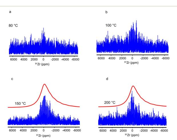
Fig. 6 Experimental 1D  $^{91}$ Zr WURST-QCPMG NMR spectra (in blue) of UiO-67-NH $_2$  submitted to steam flow during 24 h at (a) 80, (b) 100, (c) 150 and (d) 200  $^{\circ}$ C recorded under static conditions at  $B_0=18.8$  T and 140 K along with their simulated envelope (in red).
