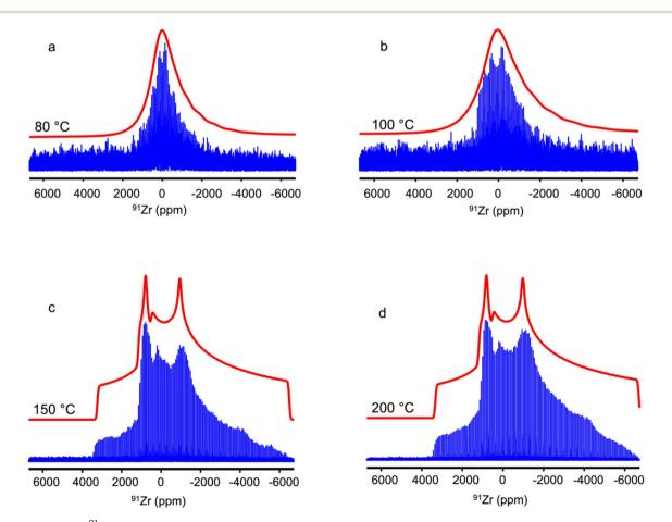
Fig. 5 Experimental 1D  $^{91}$ Zr WURST-QCPMG NMR spectra (in blue) of UiO-66-Fum submitted to steam flow during 24 h at (a) 80, (b) 100, (c) 150 and (d) 200 °C recorded under static conditions at  $B_0 = 18.8$  T and 140 K along with their simulated envelope (in red).
