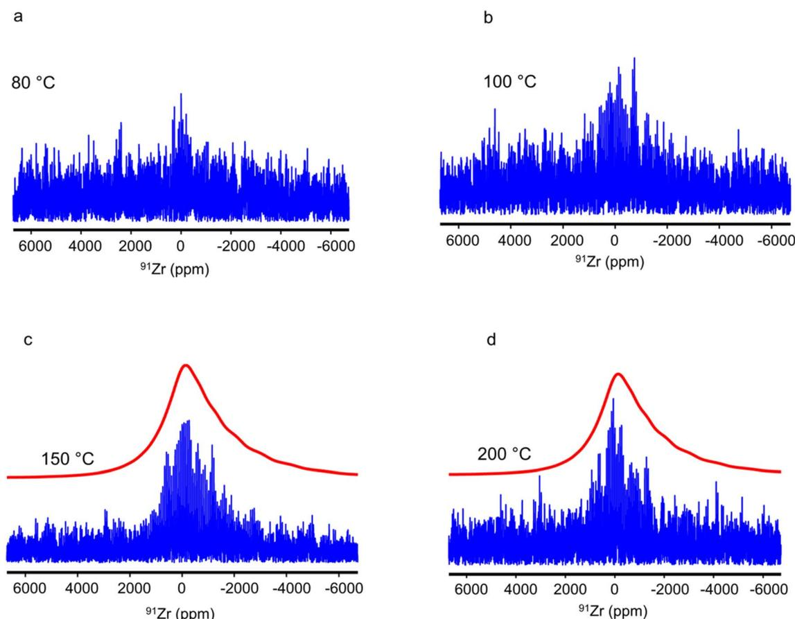
Fig. 6 Experimental 1D  $^{91}\text{Zr}$  WURST-QCPMG NMR spectra (in blue) of UiO-67- $\text{NH}_2$  submitted to steam flow during 24 h at (a) 80, (b) 100, (c) 150 and (d) 200 °C recorded under static conditions at  $B_0 = 18.8$  T and 140 K along with their simulated envelope (in red).
