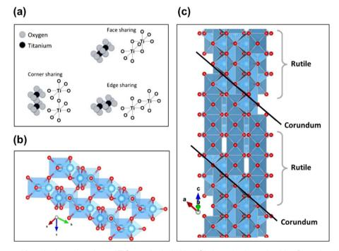
Fig. 5 (a) Edge, corner and face sharing orientations of  $TiO_2$  octahedra in Magnéli phase titanium suboxides. Reproduced with permission from ref. 23. Copyright 2010, Elsevier. (b) Corundum  $Ti_2O_3$  viewed parallel to the c axis and (c) structure of  $Ti_4O_7$ , showing four-unit rutile chains along the c direction bounded by corundum structures restricted in the (001) planes. Blue spheres represent the Ti atoms while the smaller red spheres represent O atoms.<sup>67</sup>
