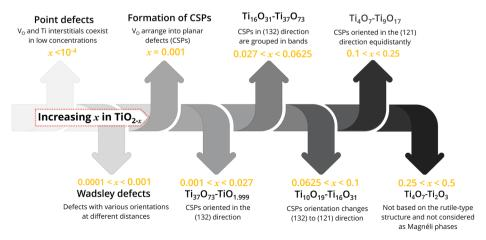
Fig. 3 Formation of different defect induced  $TiO_2$  and phases with increasing x in  $TiO_{2-x}$ .
