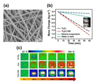
Fig. 21 (a) SEM image of fibrous  $Ti_4O_7$  membrane after calcination. (b) Rate of water evaporation from the  $Ti_4O_7$  membrane with and without YSZ. (c) Temperatures on the surface of water recorded for  $TiO_2$ ,  $Ti_4O_7$  and  $Ti_4O_7/YSZ$  membranes by an IR thermometer. Reprinted with permission from ref. 229. Copyright 2022, American Chemical Society.
