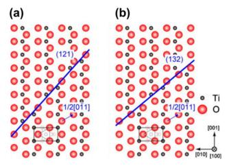
Fig. 4 Crystallographic shear structure of Magnéli phase titanium suboxides showing the shear plane formation along the (a) (121) plane and (b) (132) plane. Reprinted with permission from ref. 63. Copyright 2010, AIP Publishing.
