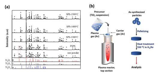
Fig. 13 (a) XRD patterns of raw powder, FSPS sample and samples prepared by conventional SPS at different temperatures. 153 (b) Preparation of TiO<sub>x</sub> nanoparticles using radiofrequency (RF) induction thermal plasma method (left) and heat treatment of the samples after synthesis to improve their electrical conductivity (right).13
