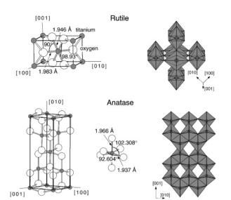
Fig. 1 Bulk structures of rutile and anatase TiO<sub>2</sub>. Reproduced with permission from ref. 11. Copyright 2003, Elsevier.
