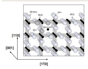
Fig. 2 Ball and stick model of the rutile  $TiO_2$  (110) surface. Large grey balls represent oxygen atoms and small black balls represent titanium atoms. Two types of point defects that are prevalent in rutile  $TiO_2$ , oxygen vacancies ( $O_{vac}$ ) and Ti interstitials, are shown. Reprinted with permission from ref. 51. Copyright 2003, Springer Nature.
