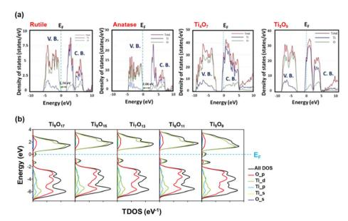
(a) Normalised DOS diagram for rutile, anatase,  $Ti_4O_7$  and  $Ti_5O_9$  (ref. 106) and (b) Calculated total DOS of Magnéli phase  $Ti_nO_{2n-1}$  ( $5 \le n \le 9$ ).
