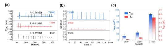
Fig. 22 (a) Measured open circuit voltage ( $V_{\rm OC}$ ) and (b) short circuit current ( $I_{\rm SC}$ ) for Magnéli phase nanocrystal films prepared at different temperatures (800–1000 °C) and (c) average peak values of  $V_{\rm OC}$  and  $I_{\rm SC}$ . Reprinted with permission from ref. 129. Copyright 2021, American Chemical Society.
