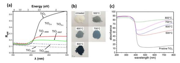
Fig. 8 (a) Diffuse reflectance spectra of  $TiO_2$  and reduced  $TiO_{2-x}$  showing the variation in light absorbance with changes in oxygen stoichiometry. Reprinted with permission from ref. 19. Copyright 2007, Elsevier. (b) Digital images of untreated and reduced rutile  $TiO_2$  and (c) UV-vis absorption (percentage scale) spectra of untreated and reduced  $TiO_2$  hydrogenated at 500-800 °C. Reprinted with permission from ref. 105. Copyright 2019, American Chemical Society.
