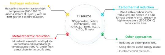
Fig. 10 Different synthesis approaches for Magnéli phase titanium suboxides (TTIP is titanium(v) isopropoxide and T<sub>x</sub> indicates functional groups) and a typical process for each method.
