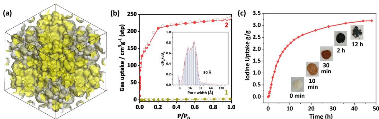
Fig. 4 (a) Accessible inner surface highlighted as yellow in a unit cell of 2. (b) The 77 K  $N_2$  adsorption isotherms of 1 and 2, and the measured pore size distribution of 2. (c) The time-dependent iodine vapor uptake performance of 2 at 75 °C under ambient pressure.
