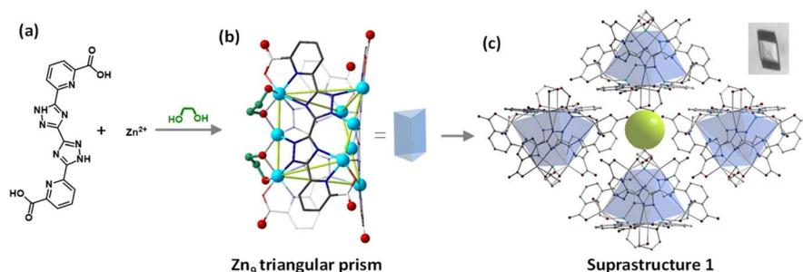
Fig. 1 Schematic representation of the synthesis and structure of supramolecule **1**: involving a ligand and metal center (a), structure view of **1** (b) and its packing mode (c), inset c is the photo of **1**. H atoms were omitted for clarity.
