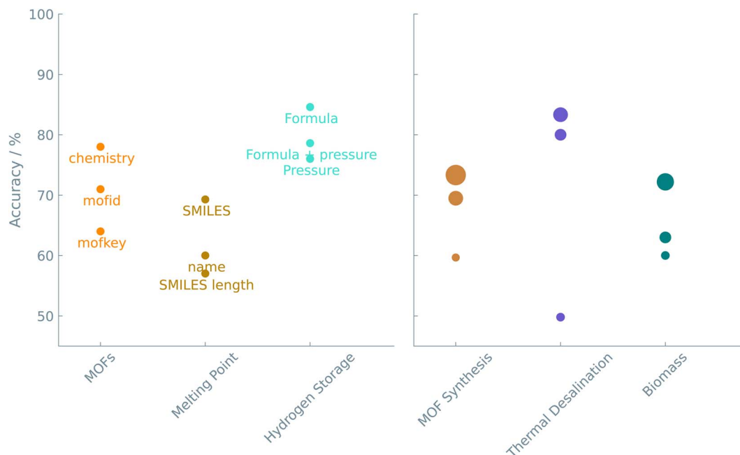
Fig. 4 Accuracy of the different representations. The color indicates the particular case study. The same color coding is used in Fig. 5 to compare between all case studies. In the left figure, the annotations are the representations used in the prompt. In the right figure, the size of the circles is related to the number of epochs used. In these examples, the results shown were obtained from fine-tuning the GPT-J model.
