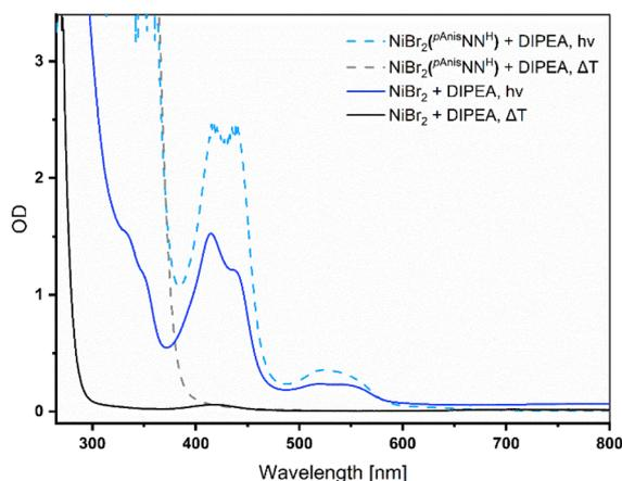
Fig. 3 UV-vis absorption spectra of  $\text{NiBr}_2$  (20 mM) with DIPEA (1.6 M, 80 equiv.) or  $6^{\text{Br}}$  with DIPEA (1.6 M, 80 equiv.) after thermal reaction at  $65\text{ }^\circ\text{C}$  ( $\Delta\text{T}$ ), and after 18 h of illumination at 455 nm (*hν*), respectively.
