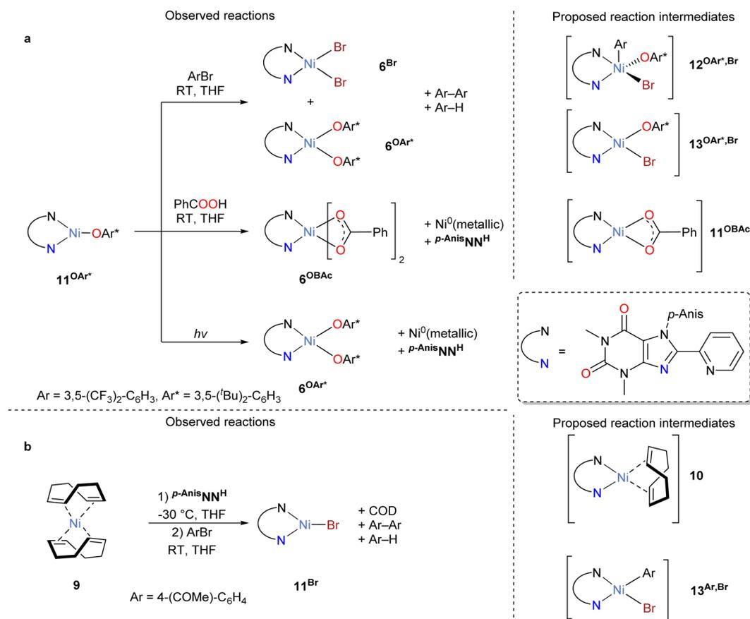
Scheme 3 (a) Oxidative addition of ArBr and transmetalation with benzoic acid from Ni(II) complex **11<sup>OAr\*</sup>** as well as decomposition from irradiation. (b) Oxidative addition of ArBr to Ni(0) complex **10**.
