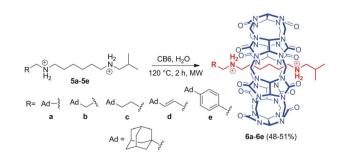
Scheme 1 Synthesis of rotaxanes 6a-6e. Counterion chlorides are omitted for clarity.
