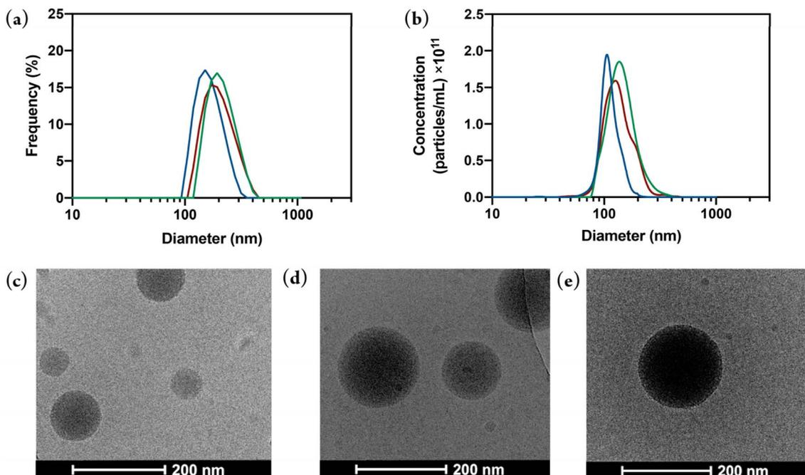
Fig. 3 Size distributions and morphology of the hybrid nanoparticles. (a) Intensity size distributions and (b) concentration size distributions of hybrid nanoparticles. 1%POM@NPs, 3.5%POM@NPs and 5%POM@NPs are shown in blue, red and green, respectively. Cryo-EM images of (c) 1%POM@NPs, (d) 3.5%POM@NPs, and (e) 5%POM@NPs. (Scale bar = 200 nm).
