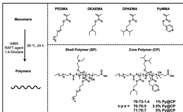
**Scheme 1** RAFT polymerization reaction scheme and structures of four different monomers, amphiphilic SP, P(PEGMA<sub>25</sub>-*b*-DEAEMA<sub>95</sub>), and three charge-shifting CPs, P(DEAEMA<sub>70</sub>-*r*-DPAEMA<sub>73</sub>-*r*-PyMMA<sub>1.4</sub>), P(DEAEMA<sub>70</sub>-*r*-DPAEMA<sub>70</sub>-*r*-PyMMA<sub>5</sub>), and P(DEAEMA<sub>71</sub>-*r*-DPAEMA<sub>73</sub>-*r*-PyMMA<sub>7</sub>). Azobisisobutyronitrile (AIBN) was utilized to initiate the polymerization.
