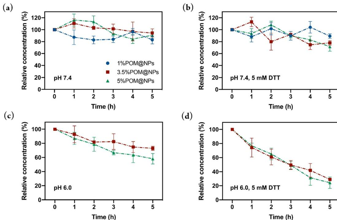
Fig. 5 pH and redox dual-induced changes in the particle concentration. The relative concentration of 1%POM@NPs (blue), 3.5%POM@NPs (red) and 5%POM@NPs (green) at pH value (a) 7.4, (b) 7.4 with addition of DTT, (c) 6.0, and (d) 6.0 with addition of DTT. Error bars represent the standard deviation of the mean, calculated from three independent replicates ( $n = 3$ ).
