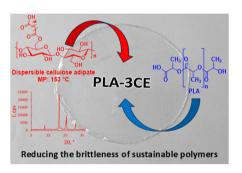
New dispersible and low-melting cellulose ester produced with molten adipic acid as a solvent, reagent and catalyst, and its application to improve the mechanical properties of PLA
