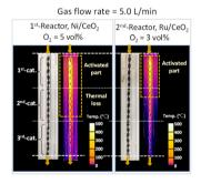
Multi-stage spiral-type structured catalyst system for direct large-scale methanation of industrial CO<sub>2</sub> emissions: a feasibility study
