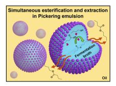
Simultaneous enzymatic esterification and ester extraction in Pickering emulsions for the recovery of butanol from fermentation broth
