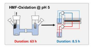
Usage of CoOOH electrodes in a flow channel reactor for the non-alkaline oxidation of 5-(hydroxymethyl)-furfural: an upscaling study
