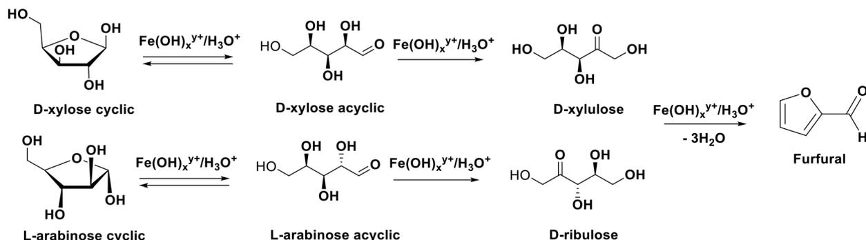
Fig. 4 Proposed mechanism for furfural formation from D-xylose and L-arabinose via isomerization and dehydration under  $[\text{Fe}_2(\text{SO}_4)_3 \cdot x\text{H}_2\text{O}]$  catalysis.
