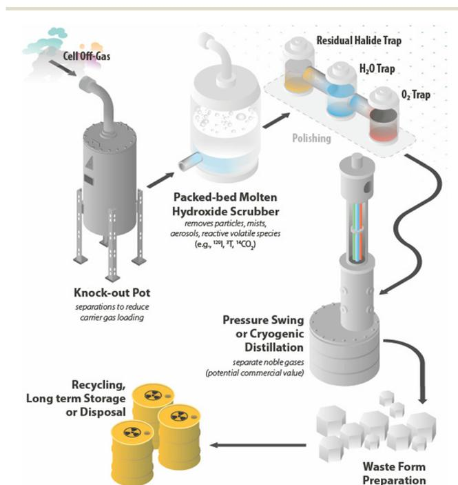
Fig. 4 Schematic of the overall off-gas system for a commercial MSR based on the MSRE experience.<sup>63</sup> All components shown, except the molten hydroxide packed-bed scrubber, are commercially available.
