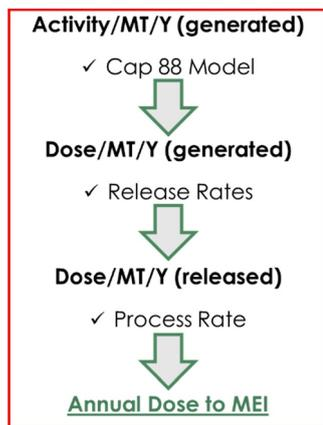
Fig. 2 Workflow illustration to determine overall dose to a maximally exposed individual (MEI).
