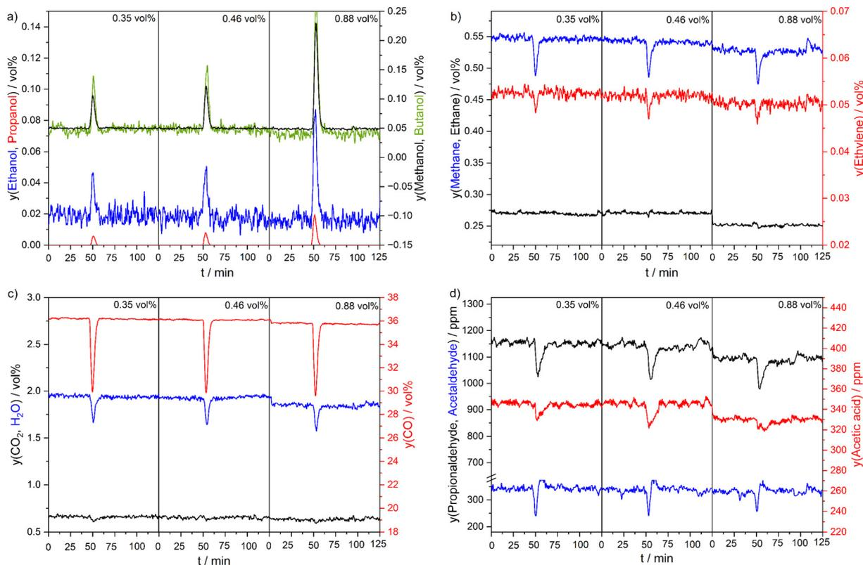
Fig. 8 Recorded mole fractions of a) the linear C<sub>1</sub>–C<sub>4</sub> alcohols, b) methane, ethane and ethylene, c) CO, CO<sub>2</sub> and H<sub>2</sub>O and d) acetaldehyde, acetic acid and propionaldehyde during the MeOH pulse series. The mole fractions of the dosed MeOH pulses are shown above the pulses.
