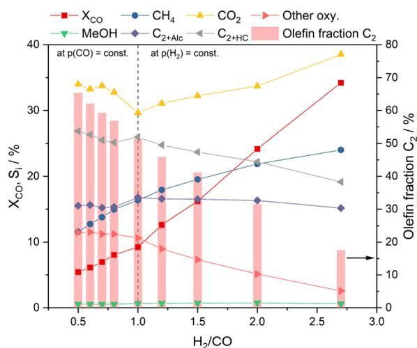
Fig. 5 Summarized selectivities and CO conversions as a function of the H<sub>2</sub>/CO ratio. The C<sub>2</sub> olefin fraction is shown as a bar diagram. The standard reaction conditions are marked with a dashed line.
