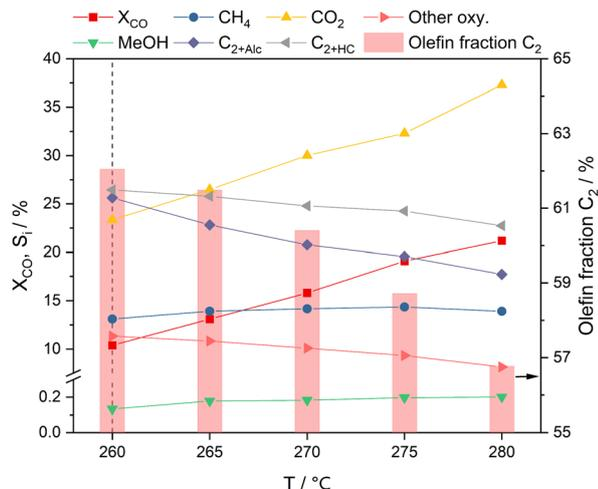
Fig. 3 Summarized selectivities and CO conversion as a function of temperature. The C<sub>2</sub> olefin fraction is shown as a bar diagram. The standard reaction conditions are marked with a dashed line.
