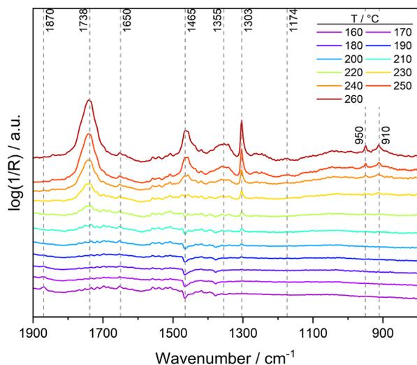
**Fig. 1** DRIFT spectra obtained during the heating phase in 20 cm<sup>3</sup> min<sup>-1</sup> syngas with a H<sub>2</sub>/CO ratio of 1 and a pressure of 60 bar.
