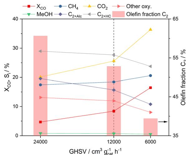
Fig. 4 Summarized selectivities and CO conversion as a function of GHSV. The C<sub>2</sub> olefin fraction is shown as a bar diagram. The standard reaction conditions are marked with a dashed line.
