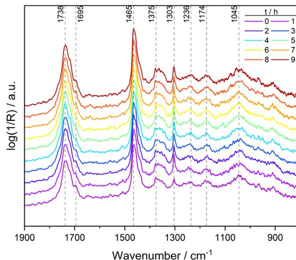
**Fig. 2** DRIFT spectra obtained during the induction period at a temperature of 260 °C, a H<sub>2</sub>/CO ratio of 1, 20 cm<sup>3</sup> min<sup>-1</sup> syngas and a pressure of 60 bar.
