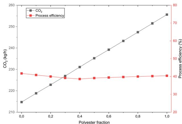
Fig. 12 Polyester fraction vs. CO<sub>2</sub> flux in off-gas and process efficiency.
