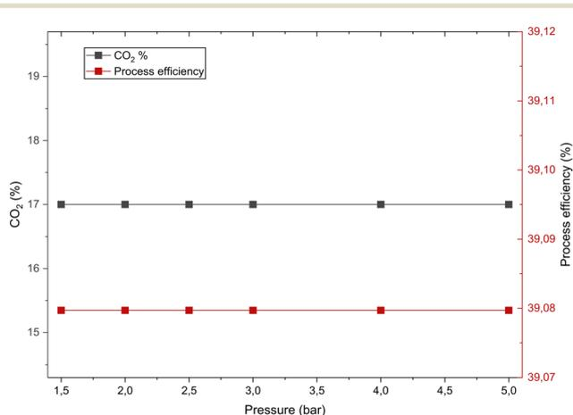
Fig. 14 Reactor pressure vs. % CO<sub>2</sub> and process efficiency (at 1000 °C).
