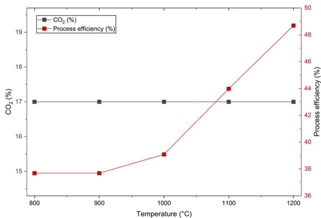
Fig. 13 Reactor temperature vs. % CO<sub>2</sub> and process efficiency (at 2 bar).
