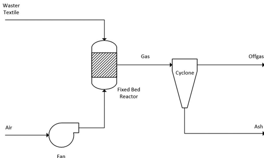
Fig. 1 Fixed bed combustion of textile waste.
