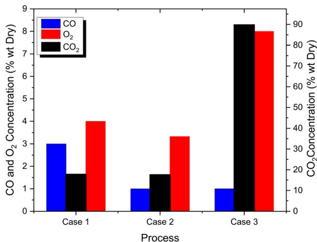
Fig. 11 Technical comparison of CO<sub>2</sub>, CO, and O<sub>2</sub> gases for reference processes (case 1) combustion (case 2) and oxy-combustion (case 3).
