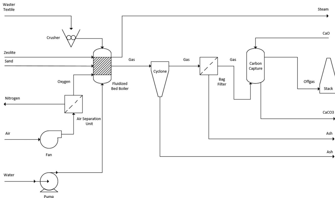
Fig. 3 Fluidized bed catalytic oxy-combustion process diagram with carbon capture.
