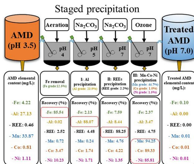
Fig. 10 Result of the integrated staged precipitation process developed for continuous AMD treatment at 150 mL min<sup>-1</sup> flow rate for Fe removal and selective recovery of Al, REEs, and Mn–Co–Ni.
