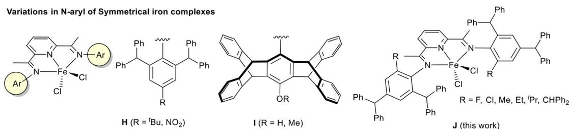
**Chart 1** Variations in the ligand structure for synthesis of high performance iron precatalysts for ethylene polymerisation.
