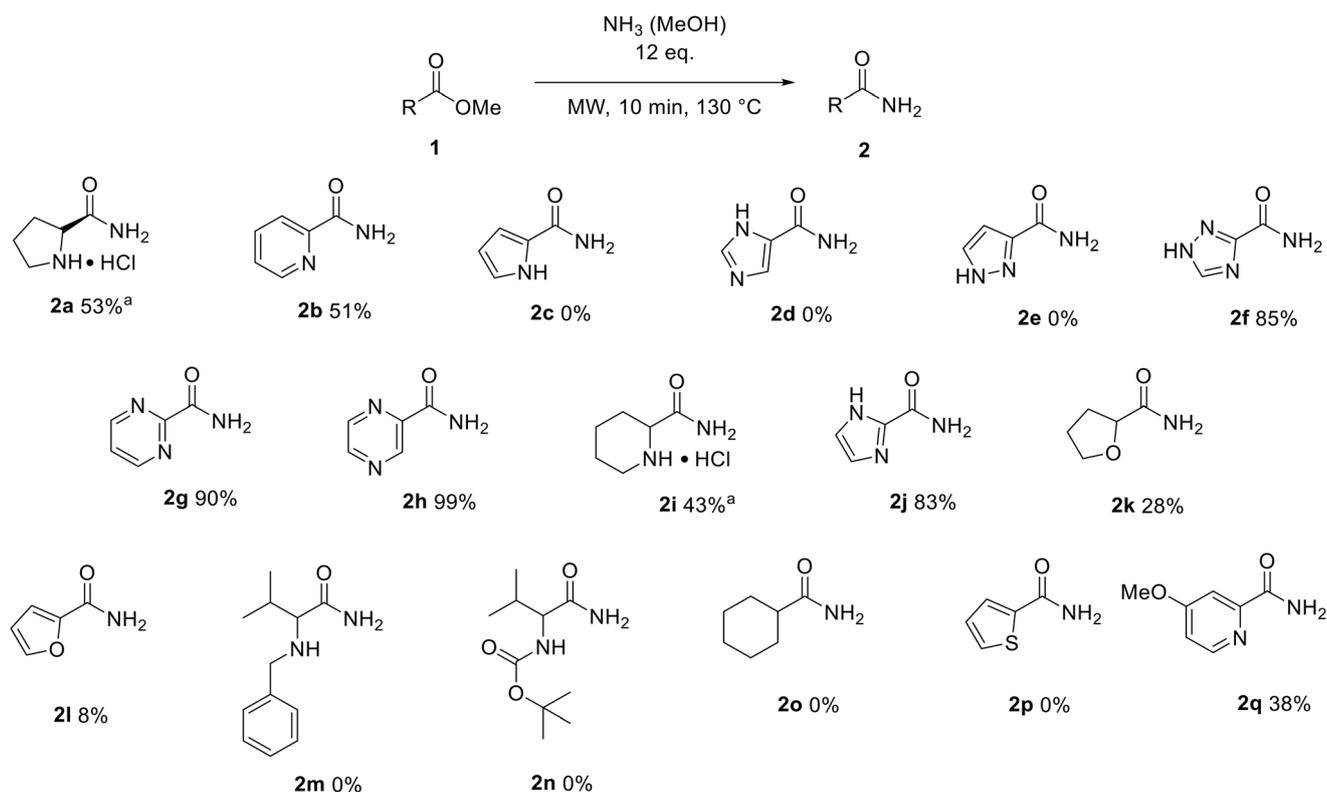
**Fig. 3** NMR yield for the ammonia-mediated aminolysis of different substrates (<sup>a</sup>methyl ester hydrochlorides are used).
