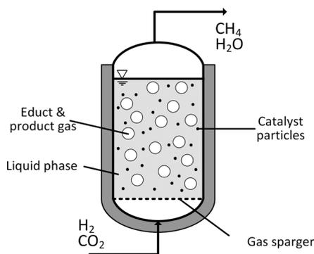
Fig. 1 Schematic drawing of a slurry bubble column reactor used for three-phase CO<sub>2</sub> methanation.
