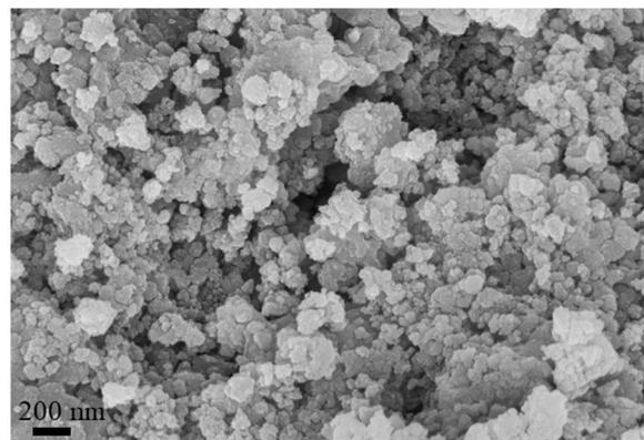
Fig. 9 SEM image of fresh reduced Ni/SiO<sub>2</sub> catalyst.
