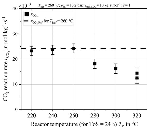
Fig. 4  $r_{\text{CO}_2}$  at  $T_{\text{Ref}} = 260$  °C after three-phase CO<sub>2</sub> methanation at different  $T_R$  for ToS = 24 h; data provided by ref. 38.
