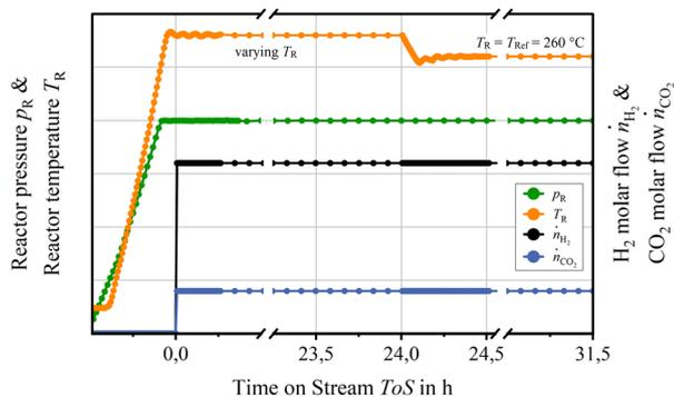
Fig. 2 Experimental procedure to determine reactor temperature that leads to catalyst deactivation.
