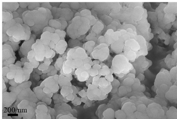
Fig. 10 SEM image of used deactivated Ni/SiO<sub>2</sub> catalyst.
