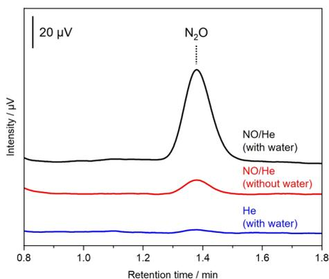
Fig. 4 GC profiles of the gases produced from different feed stocks. The catalytic tests were carried out using Pt/TiO<sub>2</sub>-pd under UV irradiation at an SV of 3500 h<sup>-1</sup>.
