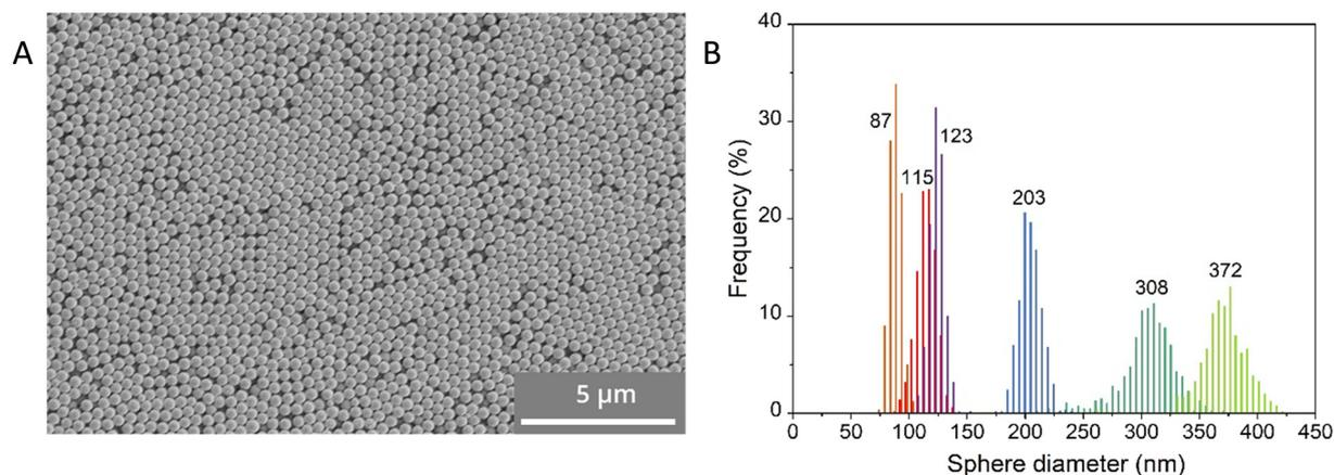
Fig. 2 A) SEM image of sample PMMA-372 showing PMMA spheres with an average diameter of 372 nm; B) diameter distributions of the PMMA spheres prepared under slightly changing reaction conditions. The numbers indicate the average diameter in nm.
