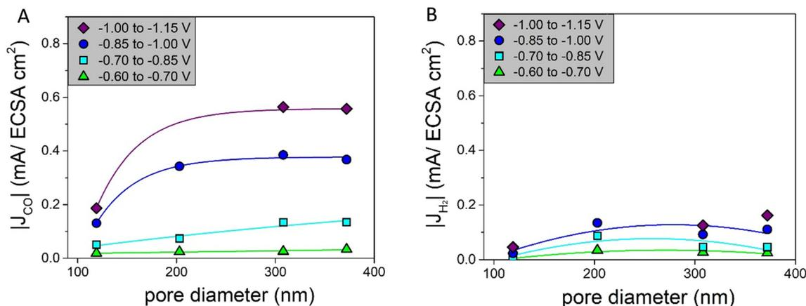
Fig. 6 A) Partial current densities of CO normalized by the ECSA for different pore diameters fitted with an asymptotic function as a line to guide the eye; B) partial current densities of H<sub>2</sub> normalized by the ECSA for different pore diameters fitted with a parabolic function as a line to guide the eye.
