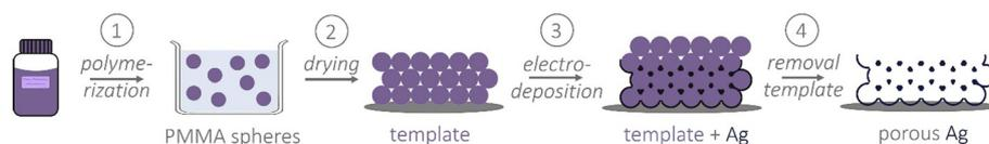
**Fig. 1** Schematic representation of the synthesis of template-based porous Ag by electrodeposition of Ag on a PMMA sphere template, involving 1) the synthesis of PMMA spheres; 2) the formation of a template on a substrate; 3) electrodeposition of Ag and 4) removal of the template. Adapted from Vink-van Ittersum *et al.*<sup>17</sup>
