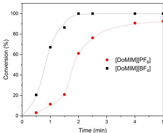
**Fig. 6** Conversion of COE to COO with various [DoMIm][X] FSAILs (X = PF<sub>6</sub><sup>-</sup>, BF<sub>4</sub><sup>-</sup>) and sodium tungstate. Reaction conditions: 50 °C, 1250 rpm, 3.7 mol% FSAIL (0.74 mmol, 3.7 equiv.), 165 mg sodium tungstate dihydrate (0.5 mmol, 2.5 equiv.), 158 mg PPA (1 mmol, 5.0 equiv.), 2.593 mL COE (20 mmol, 100 equiv.) and 1.423 mL 50 wt% aq. H<sub>2</sub>O<sub>2</sub> (25 mmol, 125 equiv.).
