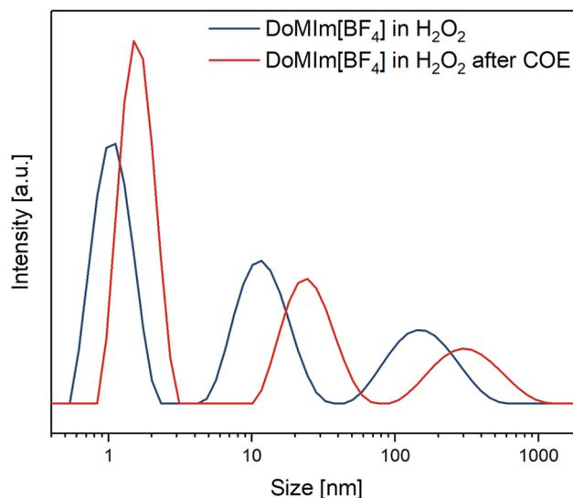
Fig. 4 DLS measurements of [DoMIm][BF<sub>4</sub>] in H<sub>2</sub>O<sub>2</sub> (357 mmol L<sup>-1</sup>) at room temperature prior and after treatment with COE.
