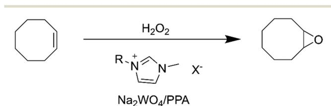
Fig. 1 General scheme of performed reactions (X = [NTf<sub>2</sub>], [BF<sub>4</sub>], [PF<sub>6</sub>]).
