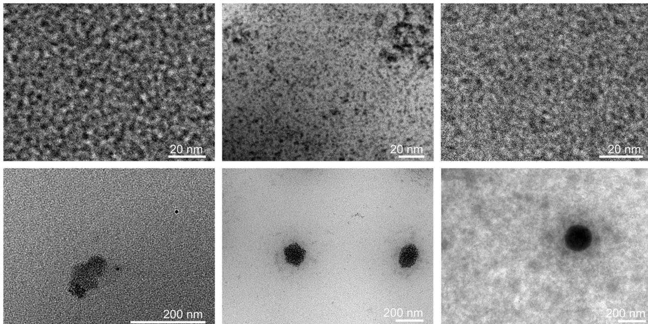
Fig. 3 Top: TEM micrographs of micelles formed by [DoMIm][NTf<sub>2</sub>] (left), [DoMIm][BF<sub>4</sub>] (middle) and [DoMIm][PF<sub>6</sub>] in saturated aqueous solutions. Bottom: TEM micrographs of micellar aggregates formed by [DoMIm][NTf<sub>2</sub>] (left), [DoMIm][BF<sub>4</sub>] (middle) and [DoMIm][PF<sub>6</sub>] in saturated aqueous solutions.
