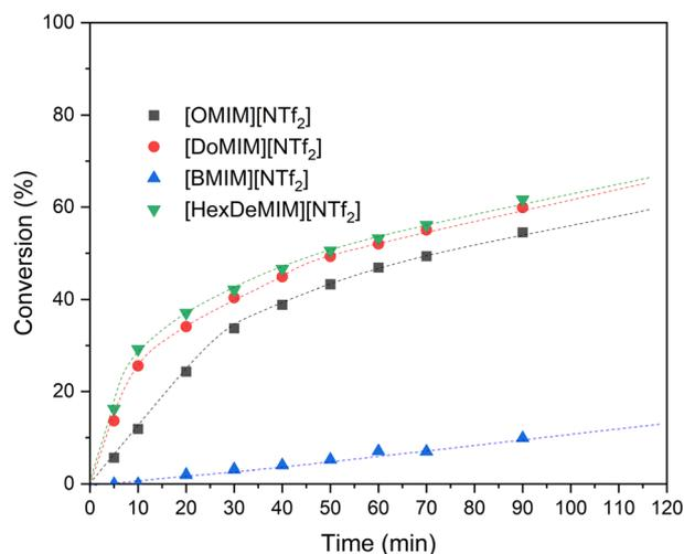
**Fig. 5** Conversion of COE to COO with different [RMIm][NTf<sub>2</sub>] SAILs (R = Bu, O, Do, HexDe) and sodium tungstate. Reaction conditions: 50 °C, 1250 rpm, 3.7 mol% SAIL (0.74 mmol, 3.7 equiv.), 165 mg sodium tungstate dihydrate (0.5 mmol, 2.5 equiv.), 158 mg PPA (1 mmol, 5.0 equiv.), 2.6 mL COE (20 mmol, 100 equiv.) and 1.4 mL 50 wt% aq. H<sub>2</sub>O<sub>2</sub> (25 mmol, 125 equiv.).
