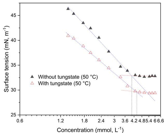
**Fig. 2** Surface tension as function of the concentration of [OMIm][NTf<sub>2</sub>] in 50% hydrogen peroxide at 50 °C with and without the addition of 18 mM of sodium tungstate. CMC values are corresponding to the dashed vertical lines.
