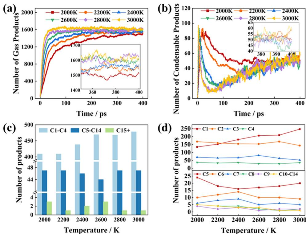
**Fig. 2** Evolution of gas (a) and condensable (b) products from xylan hydrolysis under the 2000 H<sub>2</sub> system with varying reaction times at different temperatures. Insets in (a) and (b) show magnified views of products during the late-stage reaction. (c) Variation of gas, light condensable, and heavy condensable products with changes in system temperature. (d) Variation of hydrolysis products with different carbon numbers under the 2000 H<sub>2</sub> system.
