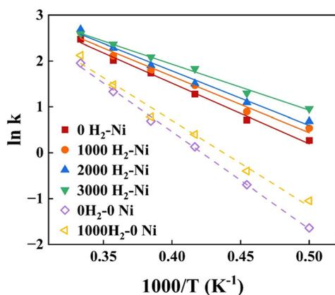
Fig. 6 The Arrhenius plot of xylan hydrolysis via ReaxFF-MD simulation.
