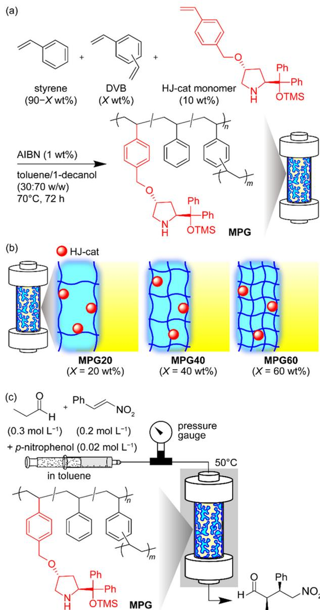
**Scheme 1** (a) Synthesis of MPG supporting HJ-cat. (b) Preparation of MPGs with different cross-linking degree. (c) Continuous-flow setup for asymmetric Michael addition of propionaldehyde to *trans*- $\beta$ -nitrostyrene.
