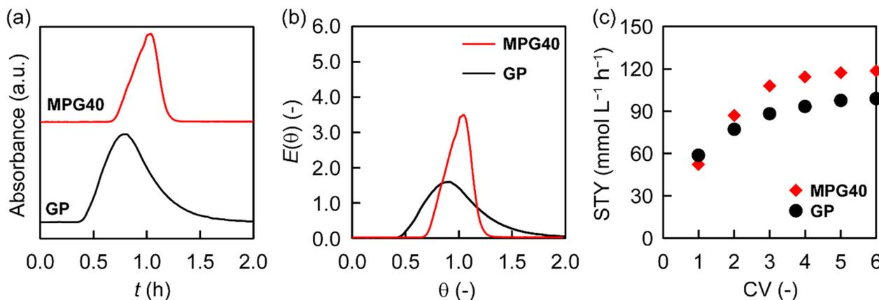
Fig. 6 (a) Elution curves and (b) dimensionless RTD curves of pulse tracers. (c) STY of **MPG40** and the **GP** in the continuous-flow Michael addition. The **MPG40** and **GP** were prepared with the same feed ratio of DVB content (40 wt%) as that for **MPG40**.
