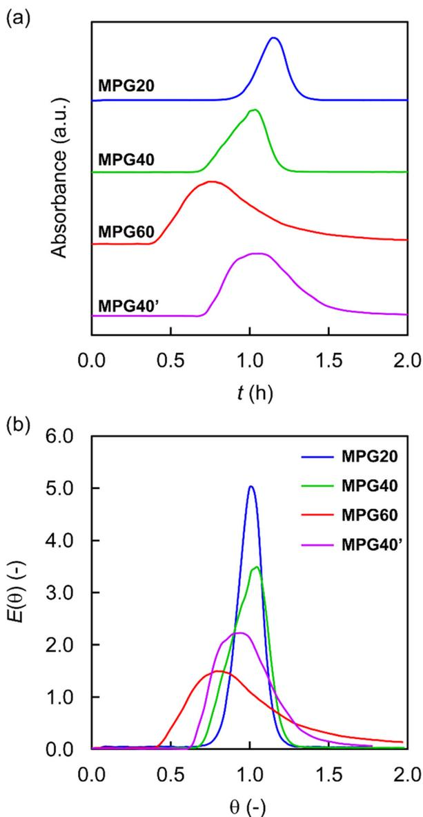
Fig. 3 (a) Elution curves and (b) dimensionless RTD curves in pulse tracer experiments for the MPG columns. Conditions: tracer = methyl red (in EtOH, 1 g L<sup>-1</sup>, 10 μL), mobile phase = toluene.
