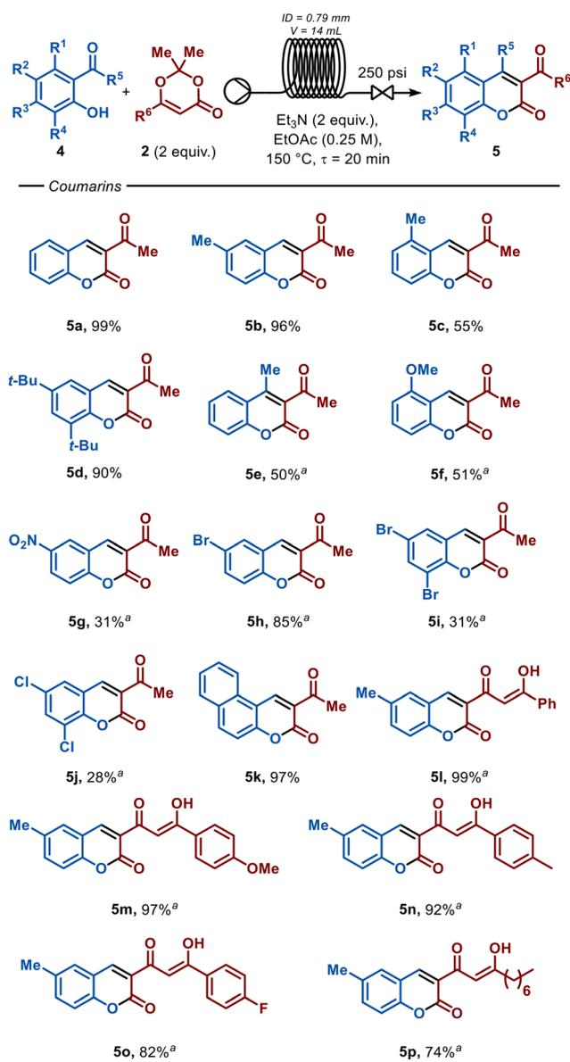
**Fig. 3** Scope of coumarins. Reaction conditions: a solution of **4** (0.50 mmol), **2** (2 equiv.), and  $\text{Et}_3\text{N}$  (2 equiv.) in  $\text{EtOAc}$  (0.25 M) was pumped at  $0.7 \text{ mL min}^{-1}$  through a 14 mL HPFA tubing (ID 0.79 mm) and heated at  $130 \text{ }^\circ\text{C}$ . Isolated yield by chromatography column. <sup>a</sup>THF used as the solvent due to poor solubility in  $\text{EtOAc}$ . NR = no reaction.
