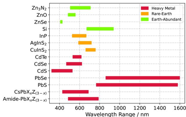
**Fig. 1** Collection of semiconductor QDs systems produced with flow-chemistry and their adjustable fluorescence emission maxima known from literature. To the best of our knowledge, a continuous synthesis process for Zn<sub>3</sub>N<sub>2</sub> QDs is evaluated for the first time in this study. It is based on non-toxic, earth abundant elements and inexpensive precursors.
