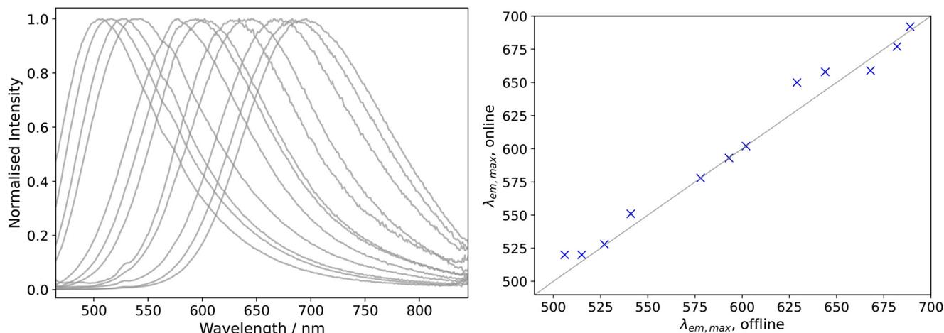
**Fig. 6** Offline fluorescence emission spectra of selected  $\text{Zn}_3\text{N}_2$  samples on the left (same samples as in Fig. 3) which highly correlate with inline measured emission peak positions as shown on the right. Consequently, integration of optical flow cells can reduce preparation time and exposure of the water/oxygen sensitive material alongside the continuous synthesis.
