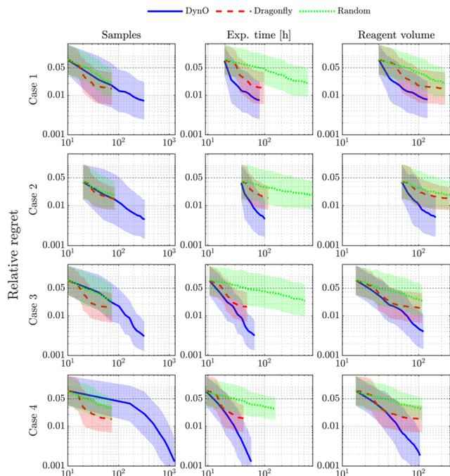
**Fig. 2** Learning curves comparing the three algorithms initialized randomly with the same data for a noise-free objective. Regret is reported as a function of number of samples, experimental time, and volume of reagents. The shaded area represents one standard deviation. A 5% regret threshold is reported as dotted line.
