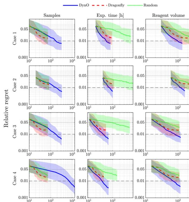
**Fig. 3** Learning curves comparing the three algorithms initialized randomly with the same data for a noisy objective. Regret is reported as a function of number of samples, experimental time, and reagents volume requirement. The shaded area is one standard deviation. A 5% regret threshold is reported as dotted line, while the 1% noise level is indicated as a dashed line.
