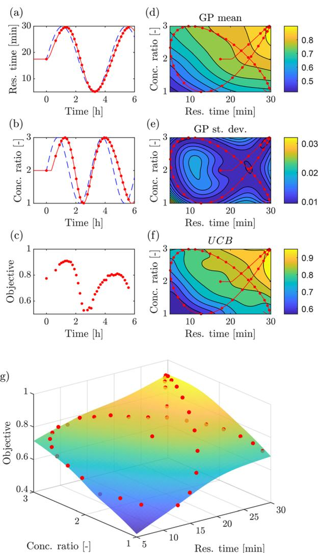
**Fig. 6** (a) and (b) Values of the optimization parameters in the initialization trajectory over time, reporting both instantaneous (dashed line) and reconstructed values (solid line). (c) Values of the objective obtained over time during initialization. Contour plots of the GP-predicted (d) objective mean, (e) standard deviation, and (f) UCB. The reconstructed initialization trajectory is drawn as a continuous line and the points are the sampled conditions. (g) GP-predictions in a 3D space.
