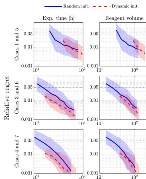
**Fig. 4** Learning curves comparing the effect of initialization (steady or dynamic) on DynO for a noise-free objective. Regret is reported as a function of number of samples, experimental time, and reagents volume requirement. The shaded area is one standard deviation. A 5% regret threshold is reported as dotted line.
