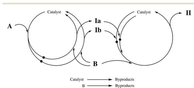
**Fig. 1** Mechanism of the reactions considered in the parametric analysis. The scheme is based on a Suzuki–Miyaura coupling of a dihalogenated species A with phenylboronic acid B, leading to three possible products. Catalyst deactivation and B degradation are also considered.
