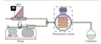
Fig. 1 Schematic representation of the experimental setup for a gasliquid continuous-flow photoreactor system, comprising a pump, mass flow controller (MFC), photoreactor system (including the reactor and light source), and a collection vessel.
