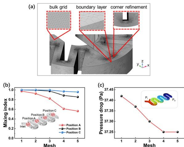
**Fig. 3** (a) Schematic diagram of the model grids. (b) The variation of the mixing index at positions A, B, and C of  $M_3$  with the number of grids. (c) The fluctuation of pressure drop at the inlet and outlet of  $M_3$  with the number of grids.
