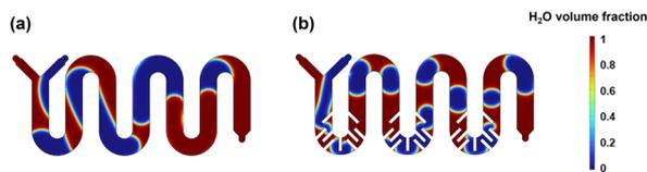
Fig. 9 Heterogeneous mixing simulation results for (a)  $M_2$  and (b)  $M_3$  (the inlet flow rate is  $2 \text{ mL min}^{-1}$ ).
