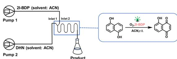
Fig. 7 Schematic diagram of the photo-oxidation reaction.
