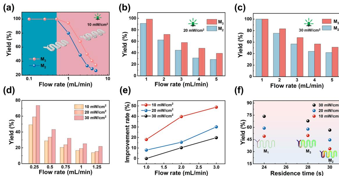
Fig. 8 Variation of juglone yield with the flow rate in different reactors. (a)  $M_2$  and  $M_3$  ( $10 \text{ mW cm}^{-2}$ ). (b)  $M_2$  and  $M_3$  ( $20 \text{ mW cm}^{-2}$ ). (c)  $M_2$  and  $M_3$  ( $30 \text{ mW cm}^{-2}$ ). (d)  $M_1$  ( $10\text{--}30 \text{ mW cm}^{-2}$ ); (e) comparison of the yield enhancement rates of  $M_3$  under different light power densities. (f) Comparison of the yields of  $M_1$ ,  $M_2$ , and  $M_3$  under different light power densities.
