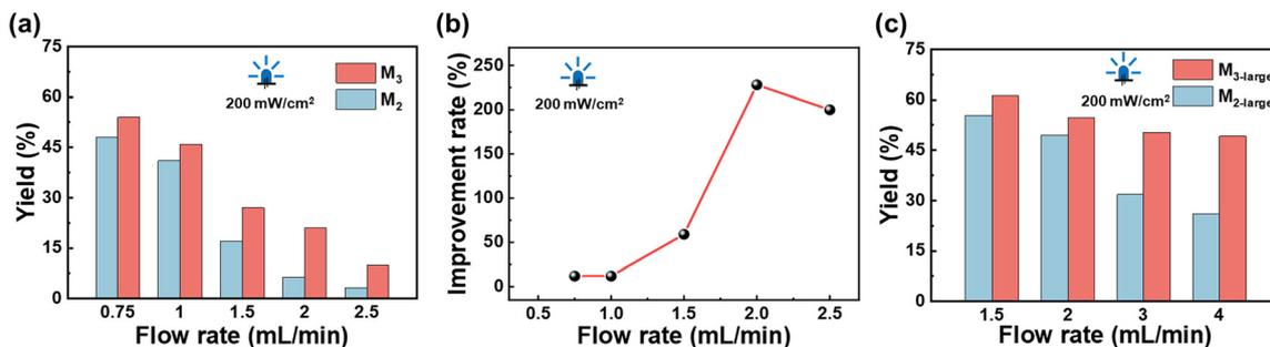
Fig. 11 (a) The yield under the same flow rate in  $M_2$  and  $M_3$ . (b) The yield enhancement rate of  $M_3$  at different flow rates. (c) The yield at the same flow rate in  $M_{2-large}$  and  $M_{3-large}$ .
