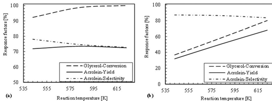
Fig. 6 Glycerol conversion, acrolein yield, and acrolein selectivity versus reaction temperature at GHSV = 1500 h<sup>-1</sup> (a) and GHSV = 8250 h<sup>-1</sup> (b) (at 1 bar reaction pressure and a mass fraction of glycerol of 0.3).
