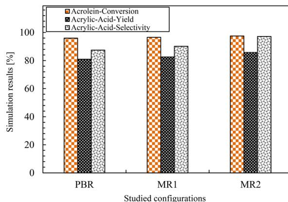
Fig. 15 Acrolein conversion, acrylic acid yield, and acrylic acid selectivity for three cases PBR, MR1, and MR2 (at temperature 583.5 K,  $GHSV$  1600 h<sup>-1</sup>, and oxygen/acrolein molar ratio of 5.7).
