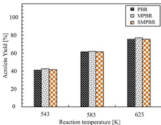
Fig. 10 Acrolein yield versus increasing reaction temperature for three cases (PBR, MBPR, and SMPBR; at 5731.6 h<sup>-1</sup>,  $P = 1$  atm and a glycerol mass fraction of 0.316).
