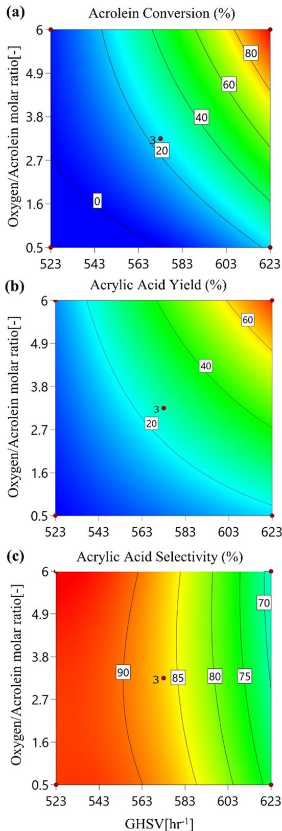
Fig. 12 Acrolein conversion (a), acrylic acid yield (b), and acrylic acid selectivity (c) versus reaction temperature at different oxygen/acrolein molar ratios (at 1 bar and a GHSV of 8800 h<sup>-1</sup>).
