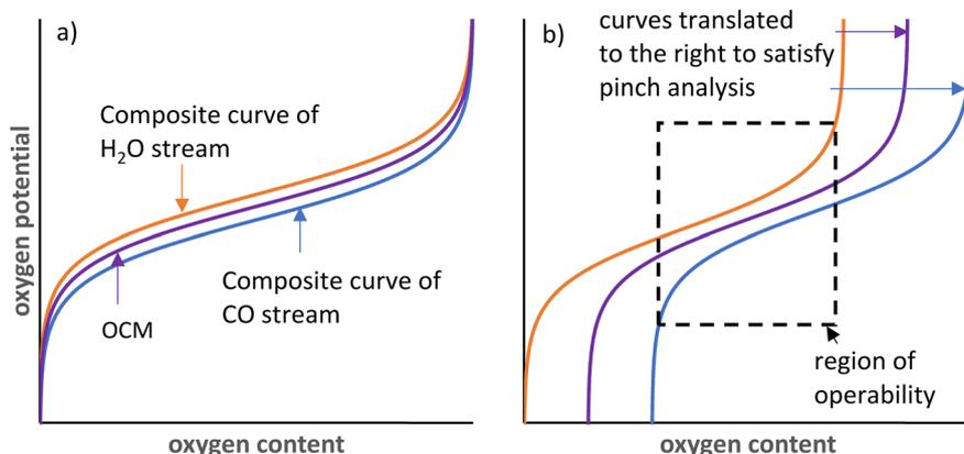
Fig. 7 Illustration of the pinch analysis for CLWGS based on an analogy to heat exchangers and composite curves. a) for cases below 1093 K and b) for cases above 1093 K. The composite curve for the  $\text{H}_2\text{O}$  stream is shown in orange, the OCM in purple and the CO stream in blue. In a) the full range of oxygen content can be utilised whereas in b), only the section within the dashed black box can be used.
