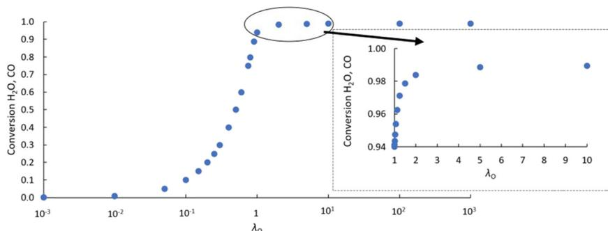
Fig. 3 Values of  $X_{\text{H}_2\text{O}}$  and  $X_{\text{CO}}$  achieved at different values of  $\lambda_{\text{O}}$  at operating temperature of 1093 K using the CLWGS reactor model. The data is taken during steady cycling where the difference between the values of  $X_{\text{CO}}$  and  $X_{\text{H}_2\text{O}}$  in successive half cycles was  $< 0.01$ . The inset shows more data points in the range  $1 \leq \lambda_{\text{O}} \leq 10$ .
