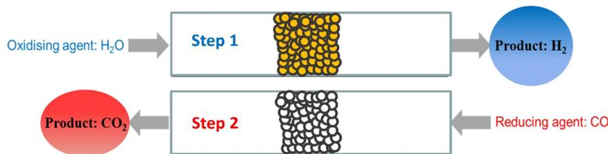
Fig. 1 A typical cycle in the CLWGS process using a packed bed reactor with a solid OCM. The bed is first oxidised by flowing through  $\text{H}_2\text{O}$ , followed by reduction in  $\text{CO}$ , flowing in the opposite direction.
