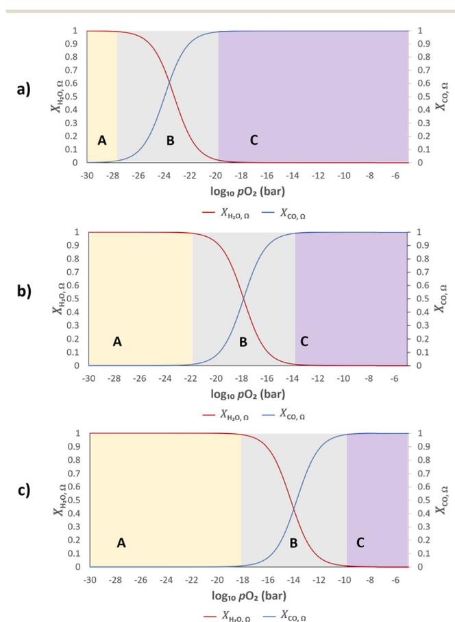
**Fig. 2** Equilibrium conversions of  $H_2O$  to  $H_2$ , and  $CO$  to  $CO_2$  as a function of  $\log_{10} p_{O_2}$ . The effect of changing temperatures at a) 893 K, b) 1093 K and c) 1293 K on the conversions is shown. Each plot is divided into regions labelled A–C, where region B represents the gas phase  $p_{O_2}$  range most relevant to the reaction equilibrium.
