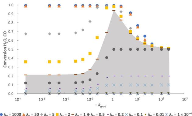
**Fig. 5** Steady state conversions determined from the simulation using different values for  $k_{\text{grad}}$  at various values of  $\lambda_{\text{O}}$ . The value of  $\log_{10} p_{\text{O}_2, \text{mid}}$  is kept constant at  $-17.8$ . The grey shaded area indicates regions where the solid phase is the limiting reactant.
