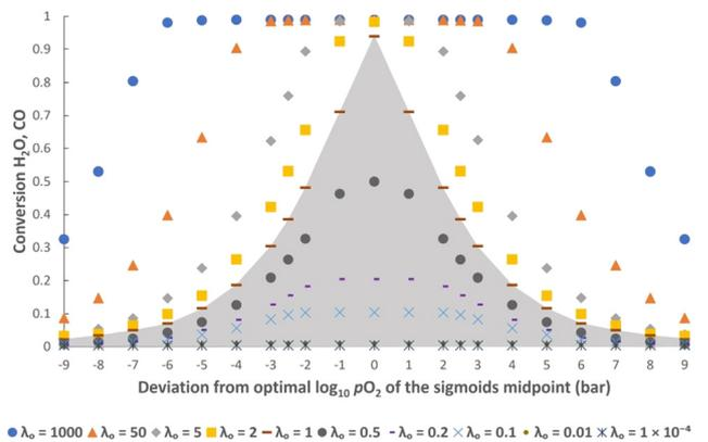
Fig. 4 Steady state conversions determined from the simulation using different values for  $\log_{10} p_{\text{O}_2, \text{mid}}$  at various values of  $\lambda_{\text{O}}$ . Midpoint values are given in reference to the deviation from the optimal midpoint of  $\log_{10} p_{\text{O}_2, \text{mid}} = -17.8$ . The value of  $k_{\text{grad}}$  is kept constant at  $-1.15$ . The grey shaded area indicates regions where the solid phase is the limiting reactant.
