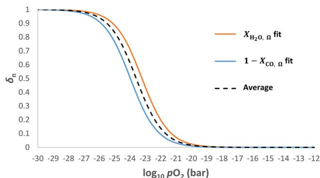
**Fig. 6** Example  $\delta_n$  vs.  $\log_{10} p_{\text{O}_2}$  profiles at  $T = 893$  K. The  $\log_{10} p_{\text{O}_2, \text{mid}}$  value of the case “average” is found by taking the average of the  $\log_{10} p_{\text{O}_2, \text{mid}}$  values for the “ $X_{\text{H}_2\text{O}, \text{O}}$  fit” and “ $1 - X_{\text{CO}, \text{O}}$  fit” cases that represent the oxidation and reduction half cycles respectively.
