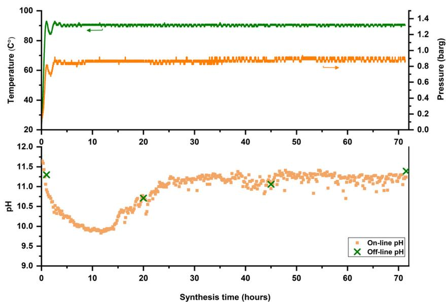
Fig. 10 Temperature, pressure, and on-line pH profiles of MFI synthesis in FB reactor. For a better comparison, *ex situ* and off-line pH measurements were also conducted during the synthesis. Molar composition of the synthesis mixtures:  $1 \text{ SiO}_2 : 0.5 \text{ TPAOH} : 32 \text{ H}_2\text{O}$ .
