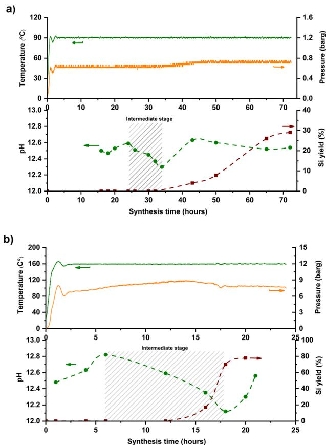
Fig. 2 Temperature, pressure, Si yield, and off-line pH profiles of MFI synthesis at (a) 90 and (b) 160 °C in FB reactor. Molar composition of the synthesis mixtures: 1 SiO<sub>2</sub> : 0.5 TPAOH : 20 H<sub>2</sub>O from TEOS as Si-precursor. The dashed line only serves as a guide to the eye. At some points, extra pH measurements without yield extrapolation were done to fully map the synthesis.
