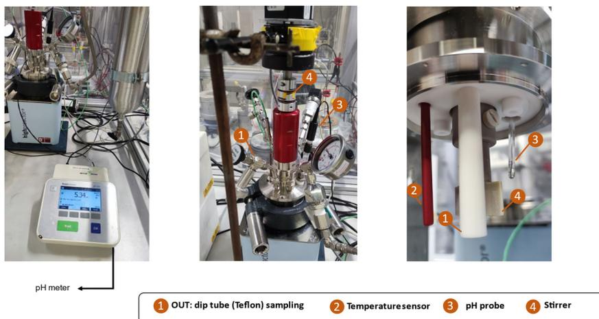
Fig. 9 The pictures of the interior and exterior of the modified FB set-up equipped with *in situ* pH probe.
