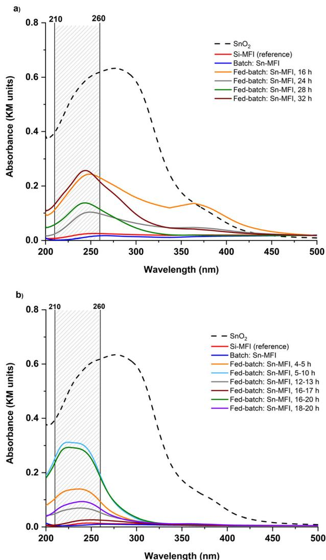
Fig. 6 Diffuse reflectance UV-visible spectra of selected (Sn-)MFI samples synthesized (a) at 90 °C and (b) 160 °C in batch and fed-batch. The materials are referenced to BaSO<sub>4</sub>. SnO<sub>2</sub> intensities were adjusted to compare fairly with other spectra.
