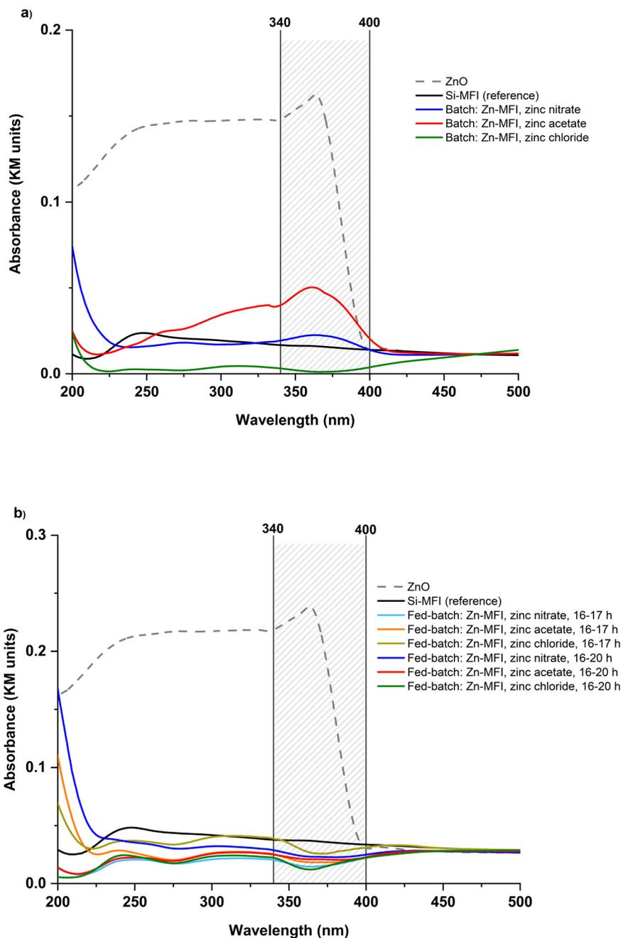
Fig. 8 Diffuse reflectance UV-visible spectra of (Zn)-MFI samples synthesized at 160 °C in (a) batch and (b) fed-batch. The materials are referenced to BaSO<sub>4</sub>. ZnO intensities were adjusted to compare fairly with other spectra.
