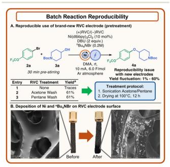
Fig. 3 Reproducibility of batch reactions. (A) Development of an electrode pretreatment to ensure reproducible data. (B) Electrode material before and after the reaction.
