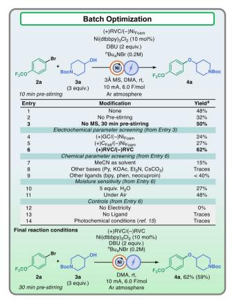
Fig. 2 Batch optimization reaction, 0.2 mmol scale. aDetermined using calibrated HPLC analysis against biphenyl as the standard. Isolated yields in brackets. Py = pyridine, bpy = 2,2'-bipyridine, phen = phenanthroline.
