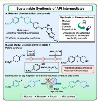
Fig. 1 Sustainable synthesis of API intermediates. (A) Delamanid, a pharmaceutical compound for multidrug-resistant tuberculosis treatment. (B) Process route towards the synthesis of intermediate 1 and the new sustainable approach.
