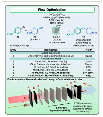
Fig. 4 Flow optimization reaction and exploded view of the flow-reactor design. Reaction scale: 1.33 mmol scale, 2.0 mmol scale with 0.1 M. <sup>a</sup>Determined using calibrated HPLC analysis against biphenyl as the standard. Isolated yields in brackets. Reactor design: (A1) inlet, (A2) outlet, (B) electrical connections, (C) graphite plate used as current collectors, (D) carbon felt electrodes, (E) PTFE gaskets, and electrode separators.
