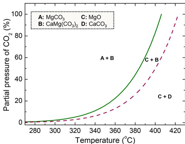
Fig. 1 Equilibrium curves of the carbonation of pure MgO (solid line) and MgO–CaCO<sub>3</sub> (dashed line) with a CaCO<sub>3</sub> to MgO molar ratio of 0.05 at 1 bar (recreated from ref. 16). In the figure, A refers to MgCO<sub>3</sub>, B to CaMg(CO<sub>3</sub>)<sub>2</sub>, C to MgO and D to CaCO<sub>3</sub>.
