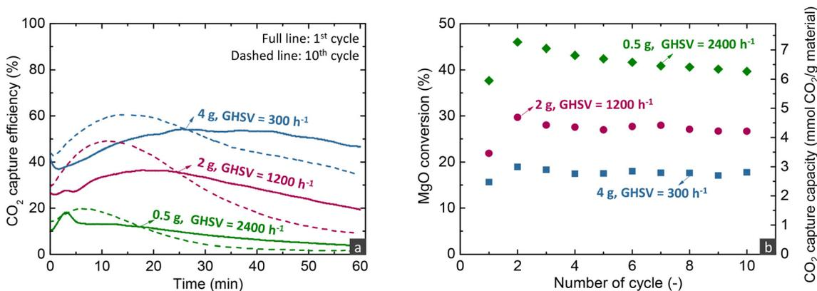
**Fig. 5** (a) CO<sub>2</sub> capture efficiency during the carbonation stage of the 1st and 10th cycles and (b) CO<sub>2</sub> capture capacity and MgO conversion over cycles for the MgCa<sub>0.05</sub>A<sub>0.20</sub> material when investigated *via* carbonate looping experiments in a fixed bed reactor with different space velocities for the carbonation stage (carbonation stage: 30% CO<sub>2</sub>/He, 300 °C; decarbonation stage: 450 °C, 100% He, 720 h<sup>-1</sup>).
