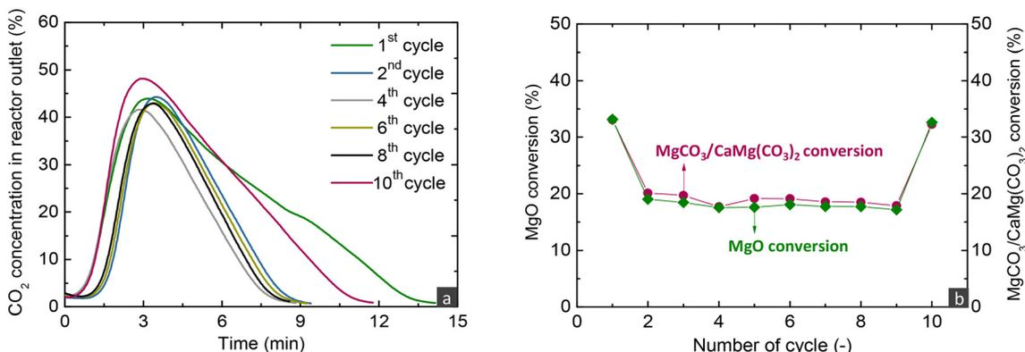
Fig. 4 (a) Outlet  $\text{CO}_2$  concentration during the decarbonation stage of different cycles and (b)  $\text{MgO}$  and  $\text{MgCO}_3/\text{CaMg}(\text{CO}_3)_2$  conversions over cycles for the  $\text{MgCa}_{0.05}\text{A}_{0.20}$  material when investigated via carbonate looping experiments in a fixed bed reactor (carbonation stage: 30%  $\text{CO}_2/\text{He}$ , 300 °C, 300  $\text{h}^{-1}$ ; decarbonation stage: 450 °C, 100% He, 720  $\text{h}^{-1}$ ).
