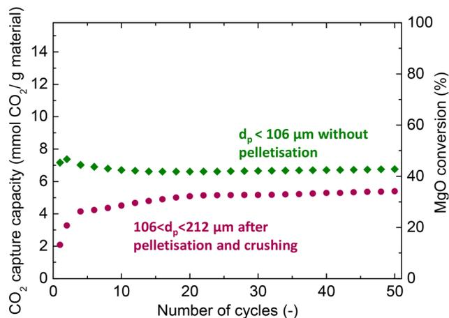
Fig. 2  $\text{CO}_2$  capture efficiency and MgO conversion for the  $\text{MgCa}_{0.05}\text{A}_{0.20}$  material obtained with and without pelletisation when investigated *via* carbonate looping experiments in a thermogravimetric analyser (carbonation stage: 30%  $\text{CO}_2/\text{N}_2$ , 300 °C; decarbonation stage: 450 °C, 100%  $\text{N}_2$ ).
