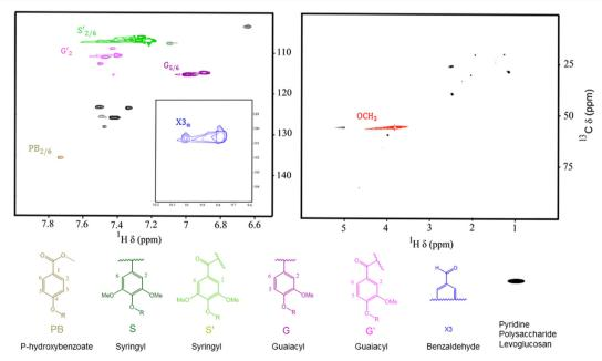
Fig. 15 HSQC NMR spectra of lignin oils obtained under alkaline oxidation conditions. Reaction conditions: 170 °C, 40 psi oxygen, 19.2 wt% catalyst, 1.25 M NaOH, 32 min.
