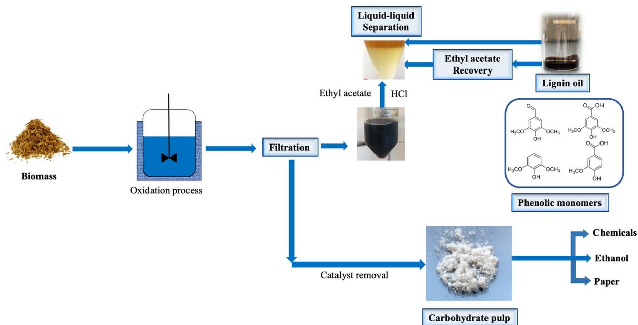
Fig. 1 Schematic diagram of the proposed integrated biorefinery process.
