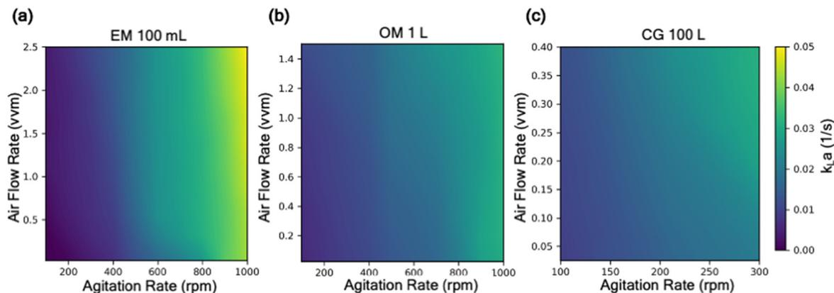
Fig. 5 Predicted  $k_La$  with varying agitation rate and air flow rate (vvm) across reactor configuration at 3 different scales: (a) 100 mL, (b) 1 L, (c) 100 L. The range of air flow rate and agitation rate in each reactor configuration is constrained by the operational limit of the reactor.
