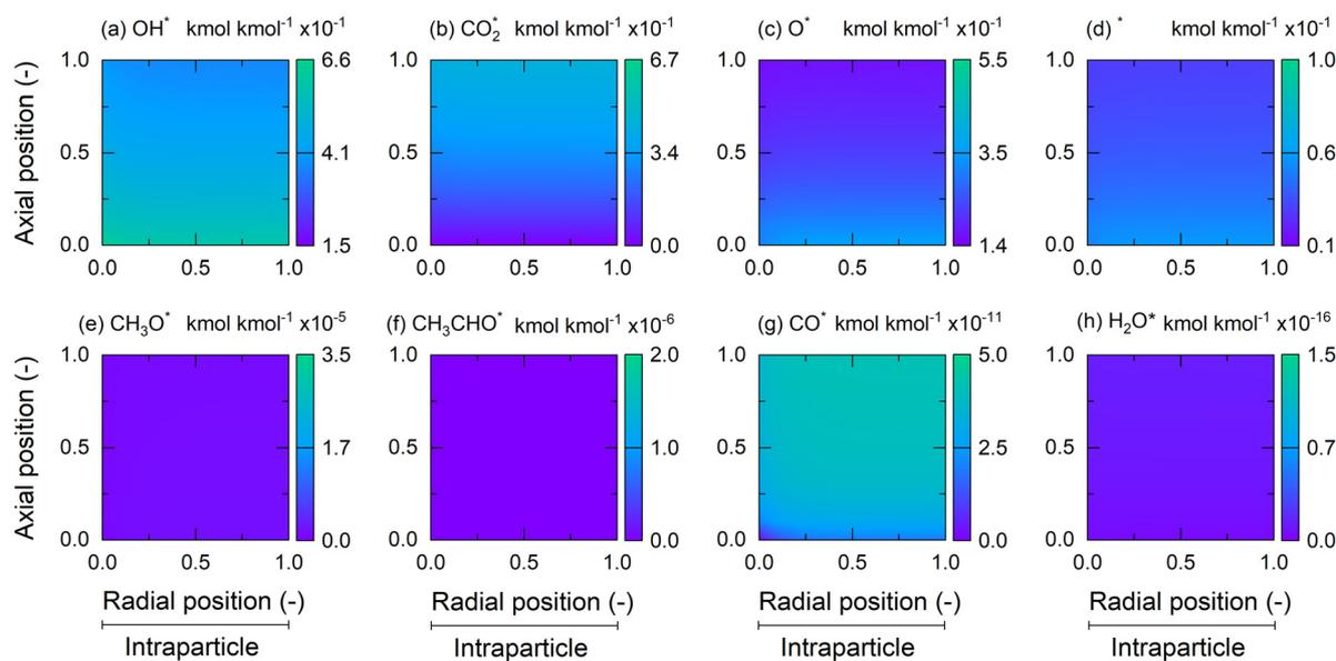
Fig. 10 Axial and radial (intraparticle phase) fractional coverage profile predictions for IMP  $\text{SiO}_2$  for (a)  $\text{OH}^*$ , (b)  $\text{CO}_2^*$ , (c)  $\text{O}^*$ , (d)  $*$  (vacancies), (e)  $\text{CH}_3\text{O}^*$ , (f)  $\text{CH}_3\text{CHO}^*$ , (g)  $\text{CO}^*$ , and (h)  $\text{H}_2\text{O}^*$ . Simulation conditions and results are identical to those of Fig. 9.
